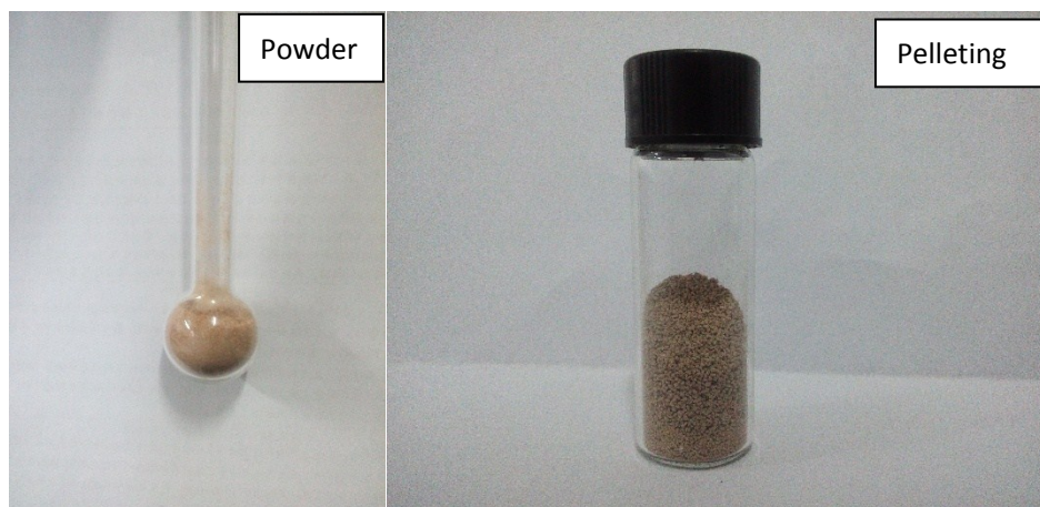
Figure S13. The powder of activated ZJU-196a and ZJU-196a after pelleting.
