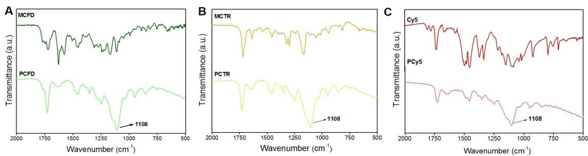
**Figure S9.** The FT-IR spectra of MCFD monomer and PCFD polymer (A), MCTR monomer and PCTR polymer (B), Cy5 and PCy5 polymer (C).
