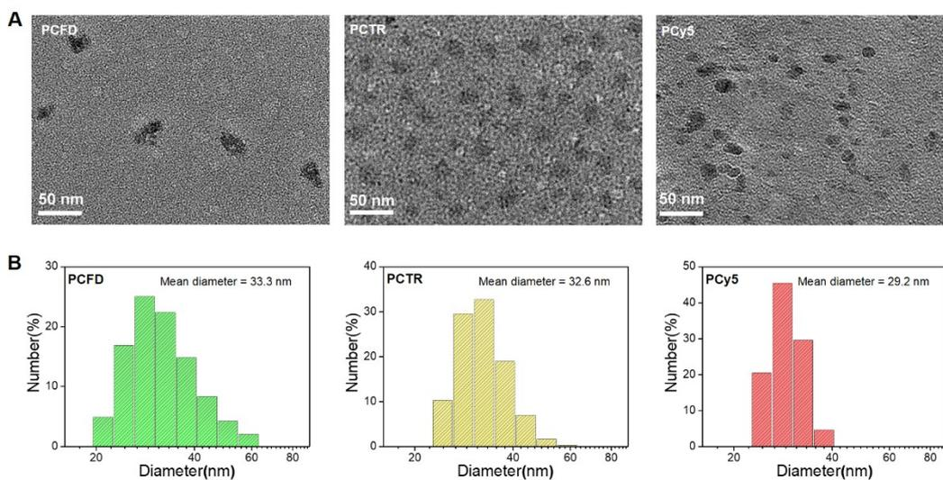
**Figure S11.** The TEM images (A) of PCFD, PCTR and PCy5 UMNs and DLS results (B) of PCFD, PCTR and  $\beta$ -CD-P(MMEA-co-OEGMA) UMNs in aqueous medium.
