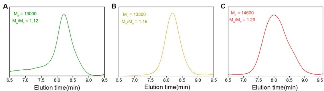
**Figure S10.** GPC traces of PCFD (A), PCTR (B) and  $\beta$ -CD-P (MMEA-co-OEGMA) (C).
