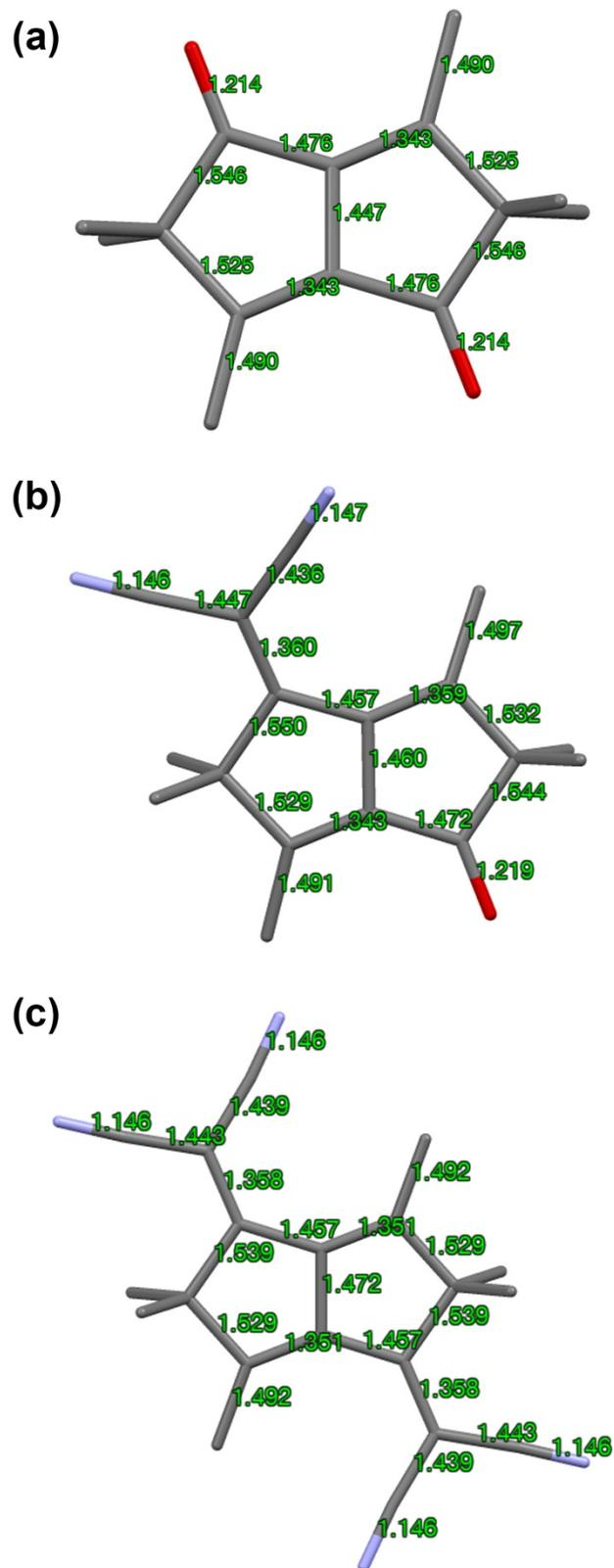
**Supplementary Figure 3.** Selected bond lengths in Å for pentalene analogues 2–4 obtained by X-ray diffraction analysis.
