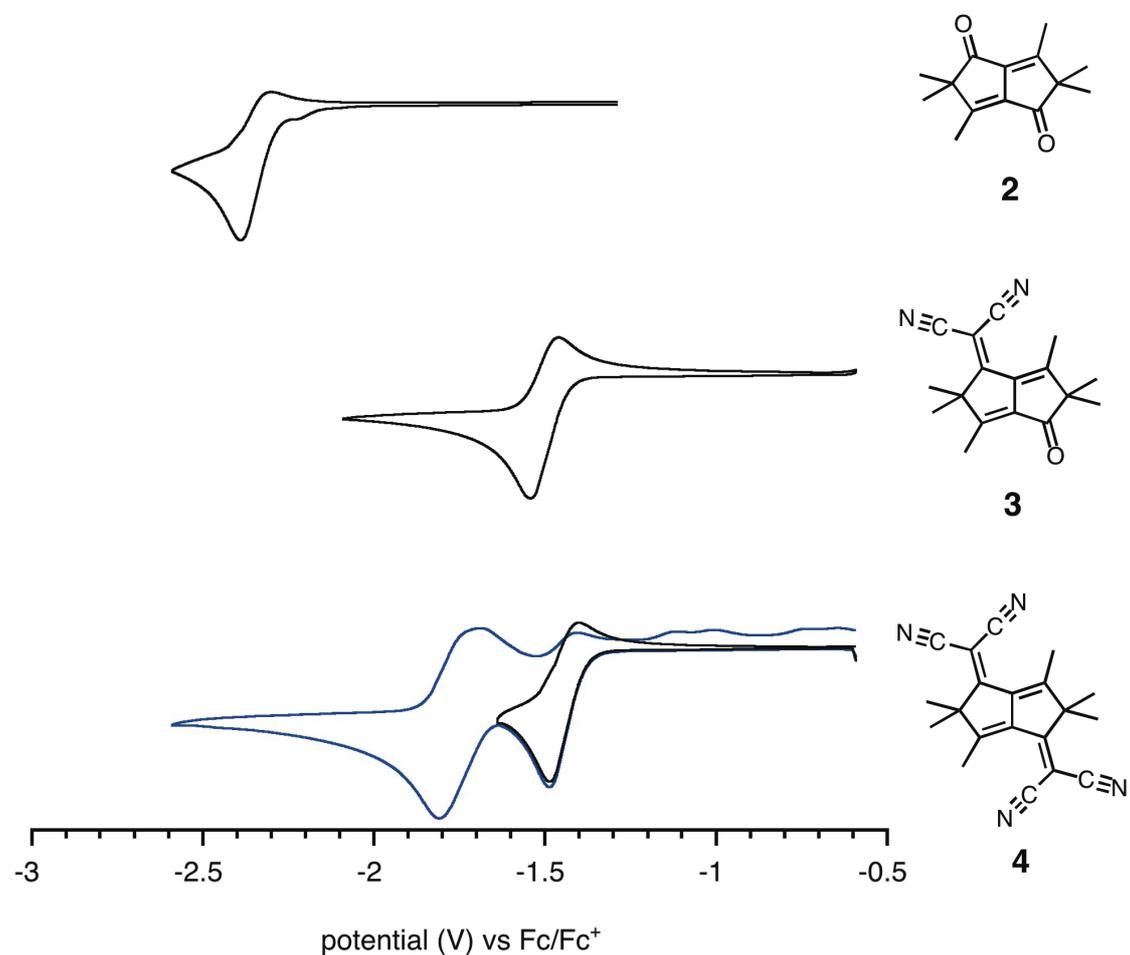
**Supplementary Figure 4.** Cyclic voltammograms of pentalene analogues **2**, **3** and **4** measured in acetonitrile at 3.0 mM using tetrabutylammonium hexafluorophosphate (10 mM) as supporting electrolyte (E/V vs. ferrocene/ferrocenium cation, scan rate 100 mVs<sup>-1</sup>).
