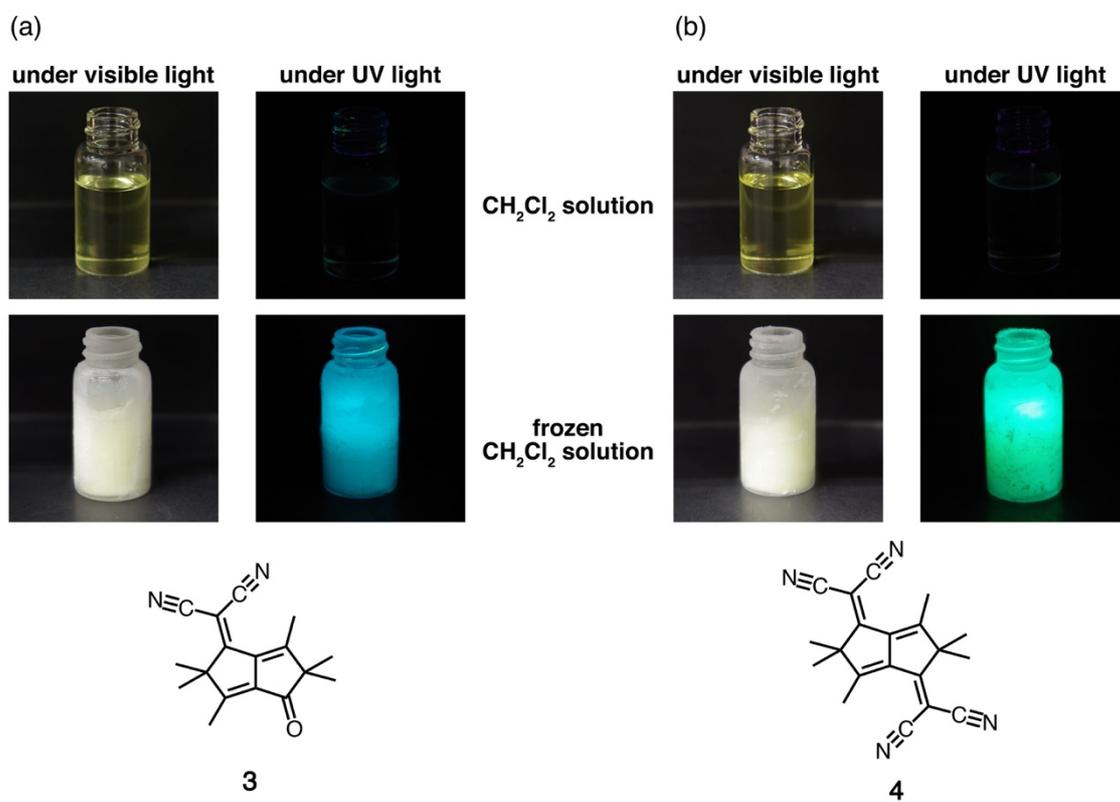
**Supplementary Figure 7.** Photographs of (top) dichloromethane solution and (bottom) frozen dichloromethane solution of compound (a) **3** and (b) **4** under visible light (left column) and UV light (365 nm) irradiation (right column).
