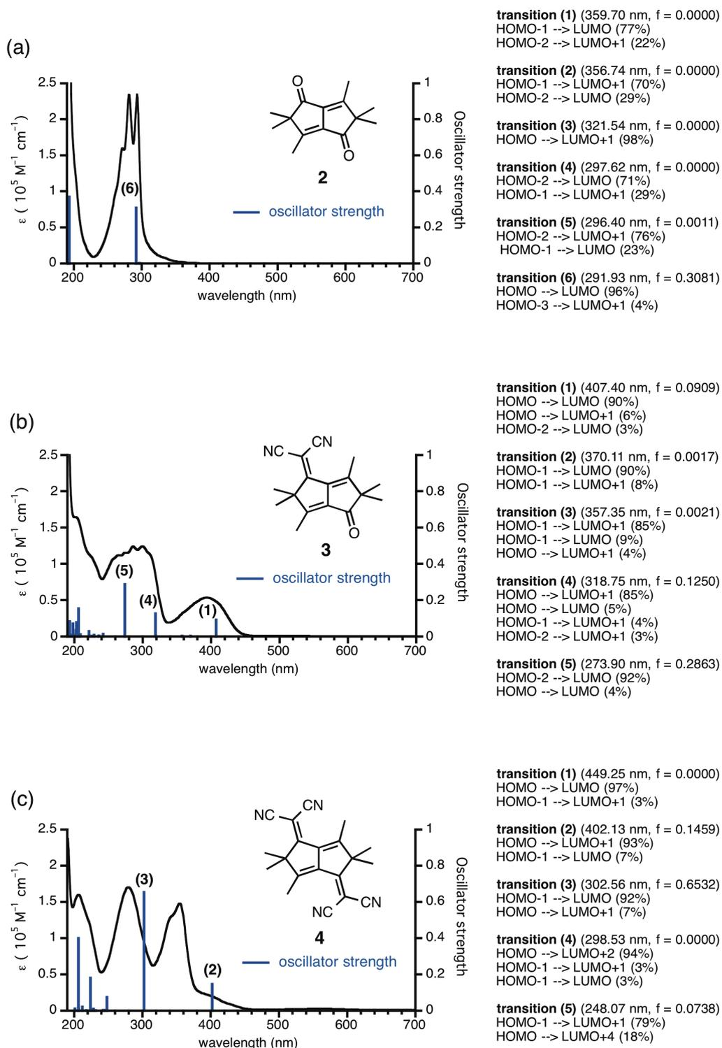
**Supplementary Figure 5.** Observed (black line) and calculated (blue bar) absorption spectra of pentalene analogues (a) **2**, (b) **3**, and (c) **4**. TD-DFT calculations were performed at the B3LYP/6-31G(d) level. Characters of several low-energy transitions were listed in the right column.
