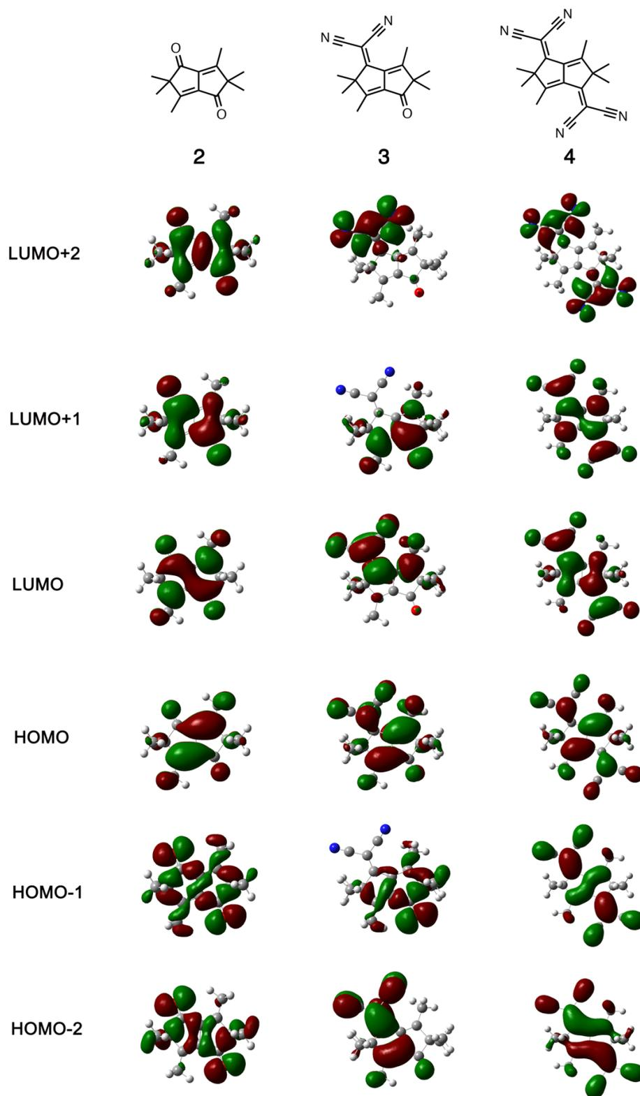
**Supplementary Figure 6.** orbital density diagrams of frontier orbitals for pentalene analogues 2–4 calculated at the B3LYP/6-31G(d) level.
