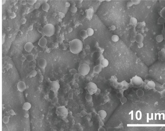
**Fig. S7** SEM image of the CM@Ni after plating 2 mA h cm<sup>-2</sup> of Li on it.
