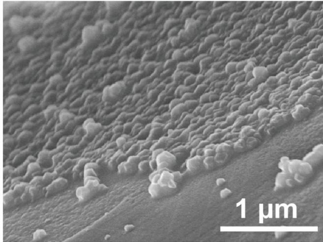
**Fig. S2** Side view SEM image of the ZIF-8@Ni.
