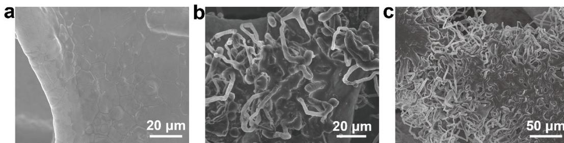
**Fig. S5** SEM images of a) the pristine Ni foam without Li plating and after plating b) 2 mA h cm<sup>-2</sup>, and c) 4 mA h cm<sup>-2</sup> of Li metal on the Ni foam.
