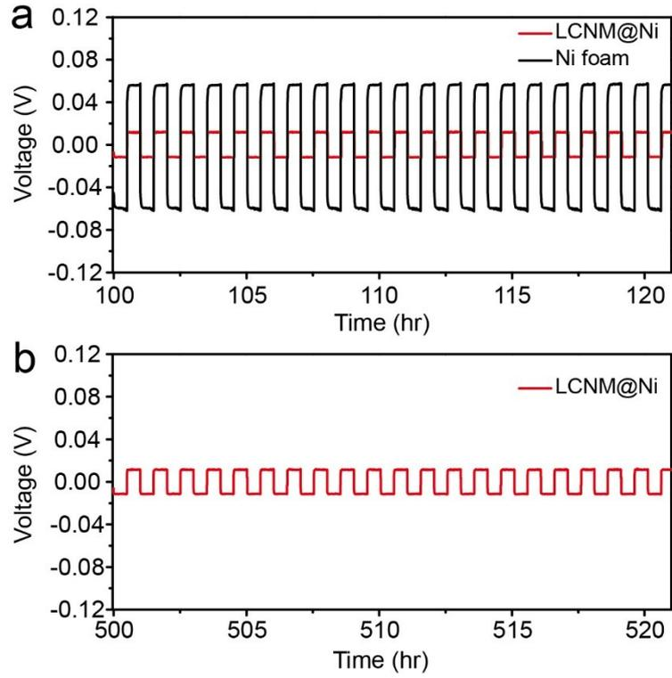
**Fig. S8** The detailed voltage profiles from a) the 100th to the 120th cycle and b) the 500th to the 520th cycle at  $2 \text{ mA cm}^{-2}$  for  $1 \text{ mA h cm}^{-2}$ .
