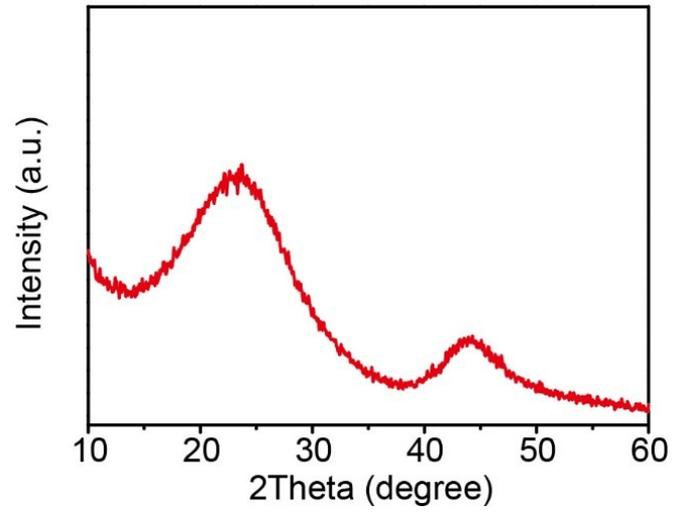
**Fig. S3** XRD patterns of the ladderlike carbon membrane.
