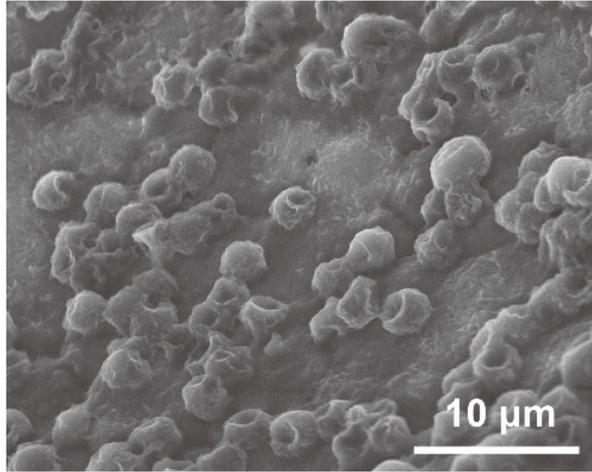
**Fig. S4** SEM image of the LCNM@Ni-Li anode after 50 cycles at the current density of  $2 \text{ mA cm}^{-2}$  and the deposition areal capacity of  $4 \text{ mA h cm}^{-2}$ .
