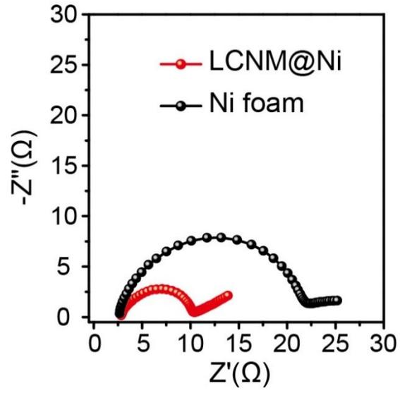
**Fig. S9** Nyquist plot of the impedance spectra of the symmetric cells before cycling at  $2 \text{ mA cm}^{-2}$ .
