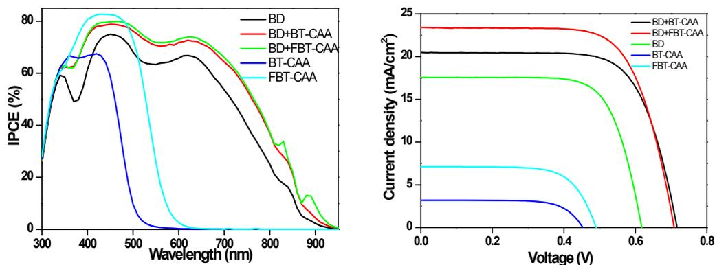
Fig-4: a) Photocurrent action (IPCE) curves of the TiO<sub>2</sub> electrodes sensitized by FBT-CAA (4a) and BT-CAA (4b), b) Current–voltage (J–V) characteristics of FBT-CAA and BT-CAA under illumination.
