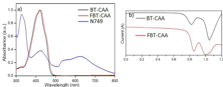
Fig-3: a) UV-visible spectra of FBT-CAA, BT-CAA and N749 in DMF solution, b) Differential pulse voltammetry (DPV) of BT-CAA, FBT-CAA
