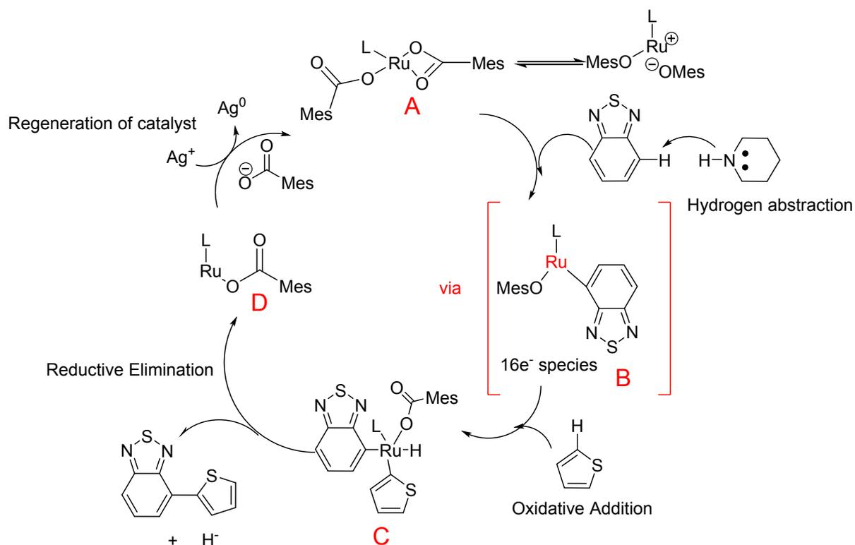
Fig-1: The Illustration of the plausible mechanism
