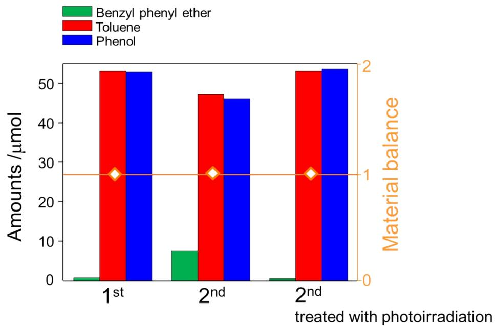
Fig. S7 Reusability of 0.5 wt% Pd-TiO<sub>2</sub> in photocatalytic cleavage of benzyl phenyl ether in a 20 vol% water containing 2-propanol solution.
