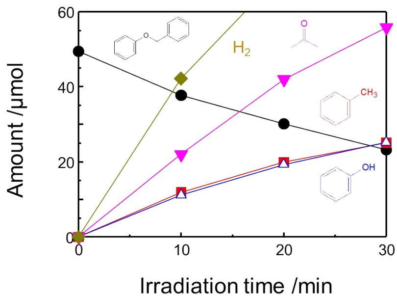
Fig. S6 Time courses of amounts of benzyl phenyl ether, toluene, phenol, acetone, and H<sub>2</sub>, during photocatalytic cleavage of benzyl phenyl ether in a suspension in 2-propanol and 0.5 wt% Pd-TiO<sub>2</sub>.
