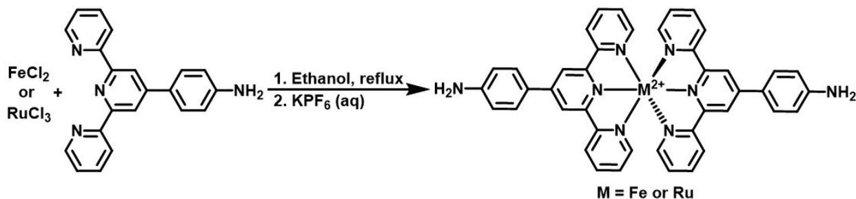
**Scheme S1.** Synthesis of  $\text{Fe}(\text{tpy-Ph-NH}_2)_2(\text{PF}_6)_2$  and  $\text{Ru}(\text{tpy-Ph-NH}_2)_2(\text{PF}_6)_2$ .
