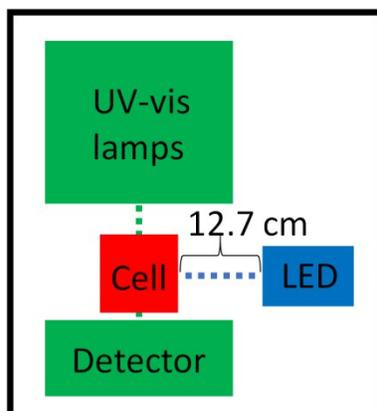
**Figure S1.** Experimental setup for kinetic measurements.
