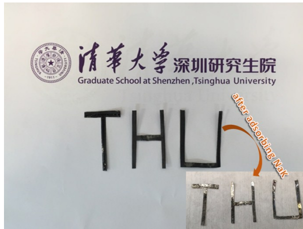
Fig. S3 Illustration of the flexible CM and CM@NaK with diverse shapes.
