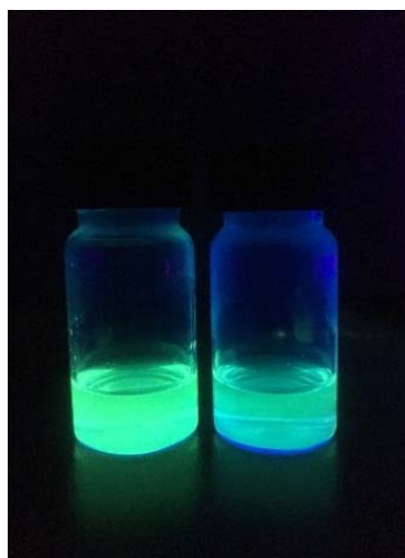
Fig. S17 Emission of the chiral imine (40 \mu M) derived from 2 and A6 in DMF (left) and 1:1 (v/v) DMF/H 2 O (right).
