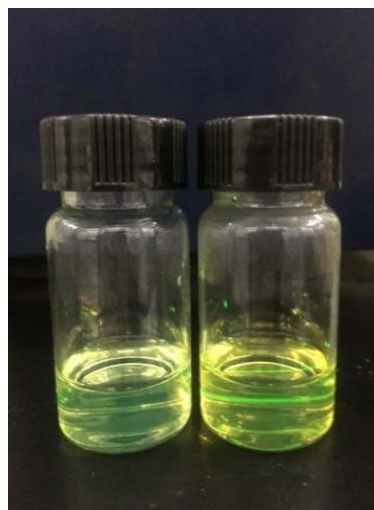
Fig. S16. Light scattering of the chiral imine (40 \mu\text{M} ) derived from 2 and A6 in DMF (left) and in 1:1 (v/v) DMF/H 2 O (right).
