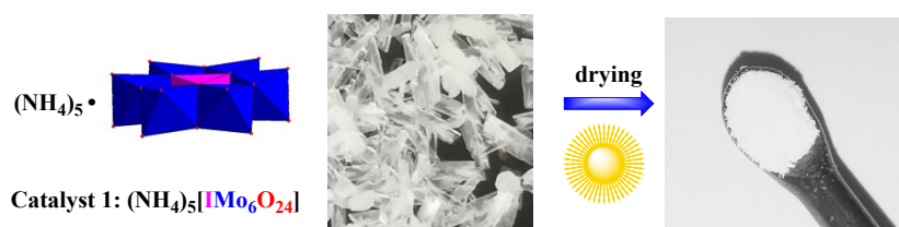
Fig. S1 Structure and appearance of (\text{NH}_4)_5[\text{IMo}_6\text{O}_{24}]
