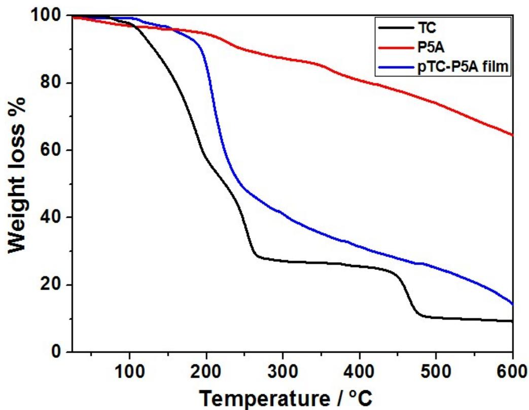
Figure S11. TGA curves for P5A (red), pTC-P5A film (blue), TC (black).
