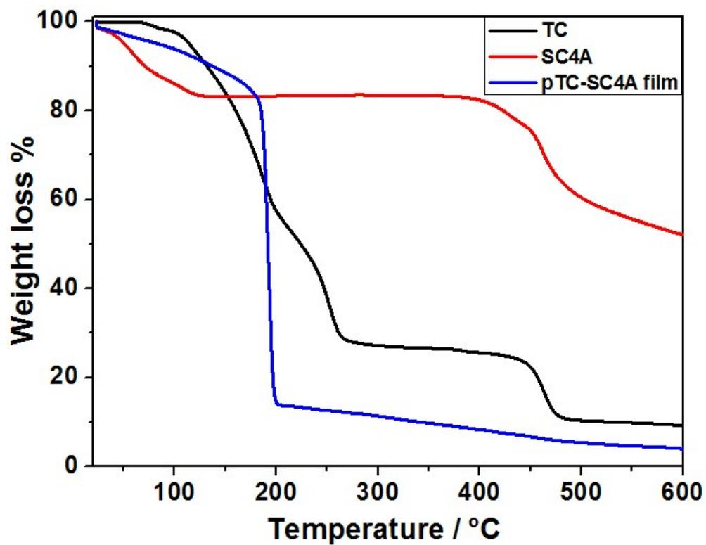
Figure S10. TGA curves for SC4A (red), pTC-SC4A film (blue), TC (black).
