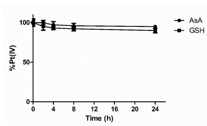
**Figure S1.** Ascorbic acid (AsA) and glutathione (GSH) reduction of **1** as analysed by HPLC. A solution of **1** (100  $\mu$ M) in PBS at 37  $^{\circ}$ C was treated with AsA or GSH to give final concentrations of 1 mM of each reductant.
