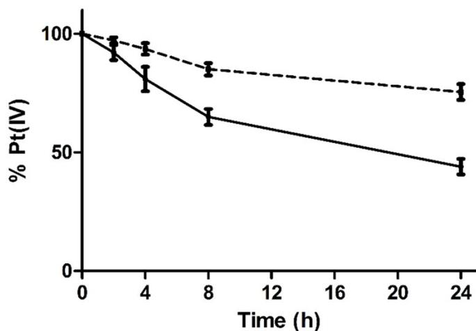
**Figure S3.** Electroactivation of **1** (100  $\mu\text{M}$ ) with the mediator (50  $\mu\text{M}$ ) in PBS (solid line) and without mediator (dashed line), as measured by HPLC. A reduction potential of -0.4 V was applied to a glassy carbon electrode vs. the Ag/AgCl reference electrode over 24 h, with samples taken at time-points for analysis.
