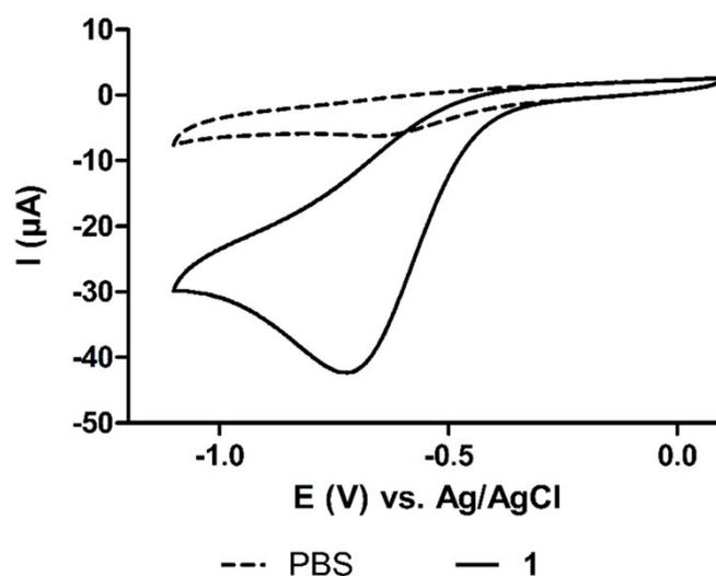
**Figure S2.** Cyclic voltammograms of PBS alone (dashed line) and a solution of prodrug **1** (2 mM) in PBS. A glassy carbon electrode was used as the working electrode, with potentials shown relative to the Ag/AgCl reference electrode employed.
