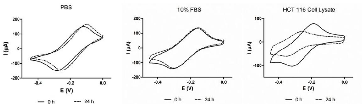
**Figure S5.** Cyclic voltammograms recorded for a modified screen-printed electrode in: (a) PBS, (b) FBS and (c) cell lysate over 24 h. Potentials are relative to the Ag pseudo-reference.”
