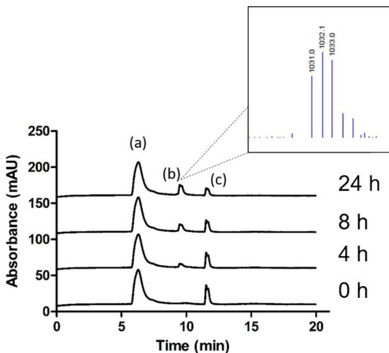
**Figure S10.** HPLC trace showing: (a) GMP, (b) Pt(II)-GMP<sub>2</sub>, (c) **1**. Inset: Analysis of peak (b) by LC-MS confirmed that DACH-Pt-GMP<sub>2</sub> was formed.
