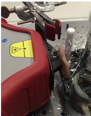
Figure S2 - Experimental set-up using a handheld SERS spectrometer for the detection of nanotags through tissue. Nanotag solutions were held in a cuvette and the cuvette was placed behind tissue samples. The nose cone was brought into contact with the tissue to ensure there was no space between the tissue sample and the instrument.
