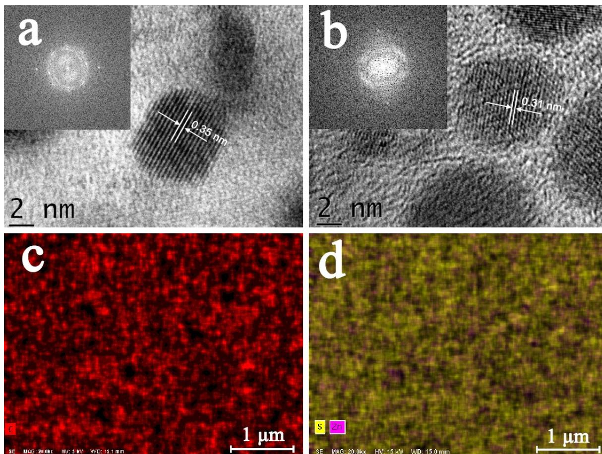
**Fig.S8** High-resolution TEM images of (a) CQDs and (b) C-ZQDs. SEM mapping of (c) CQDs at  $m\text{-TiO}_2$  film and (d) C-ZQDs at  $\text{CsPbBr}_3$  film. The inserts show the selected area electron diffraction patterns of CQDs and C-ZQDs.
