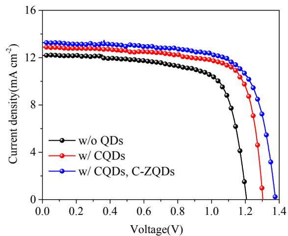
**Fig. S4** The  $J$ - $V$  curves of various solar cells with both side light illumination at a time.
