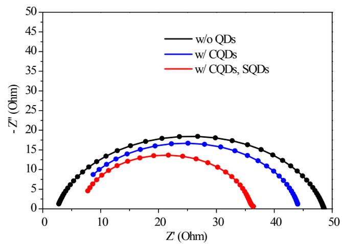
**Fig. S10** EIS Nyquist plots of three bifacial PSCs measured at open circuit in the dark.
