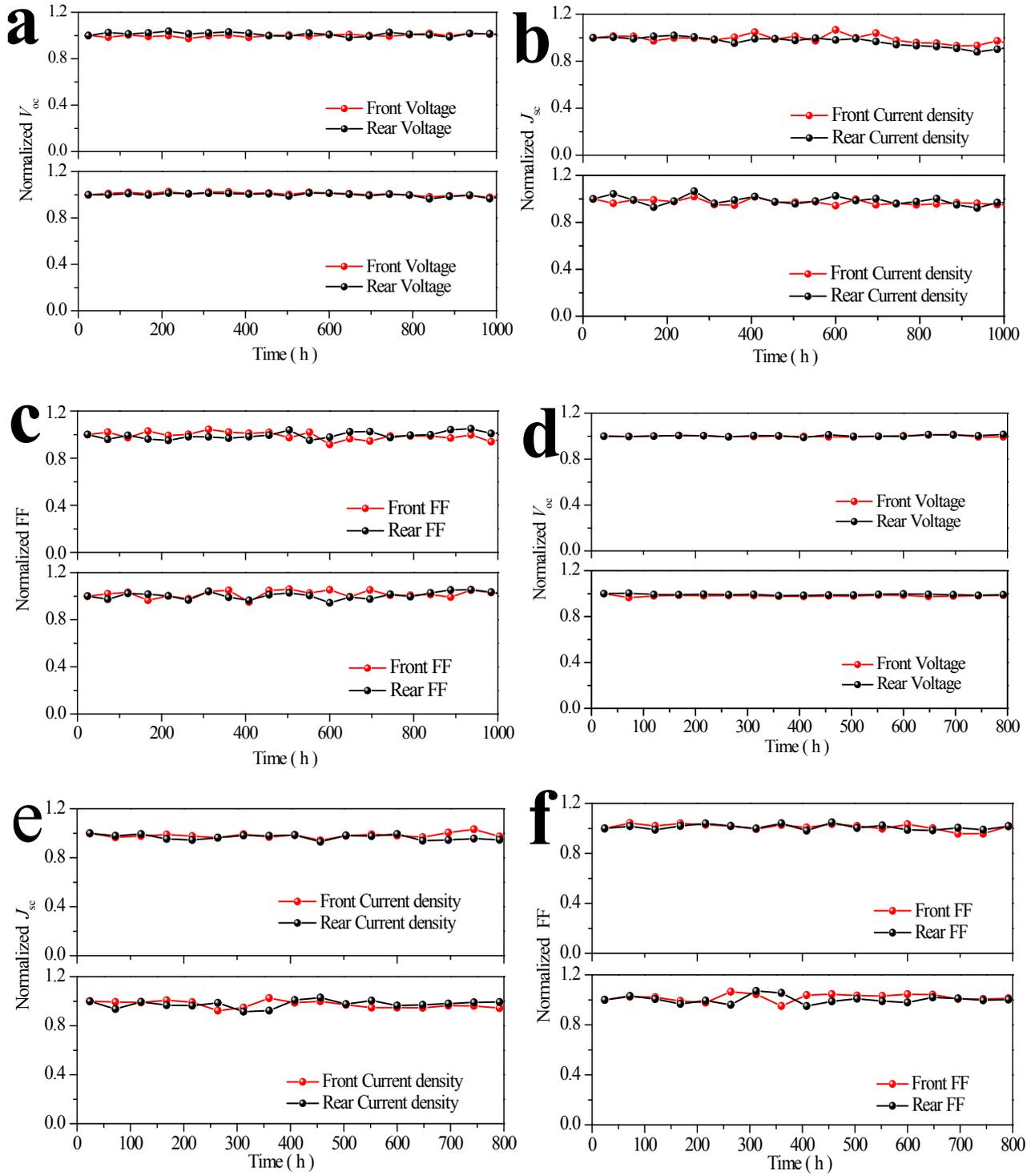
**Fig. S12** Normalized photovoltaic parameters for bifacial PSCs including (a)  $V_{oc}$ , (b)  $J_{sc}$ , (c)  $FF$  as a function of aging time at 60% RH and 25 °C. Normalized photovoltaic parameters for bifacial devices including (d)  $V_{oc}$ , (e)  $J_{sc}$ , (f)  $FF$  as a function of aging time at 80 °C.
