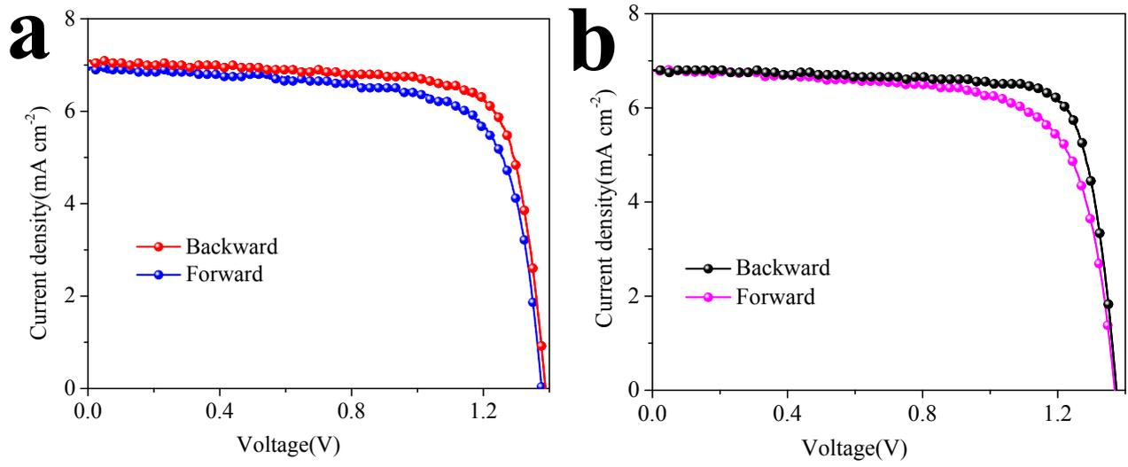
**Fig. S3**  $J$ - $V$  curves of the CQDs/C-ZQDs modified bifacial PSCs under different scan conditions: (a) upon irradiation from front side and (b) upon irradiation from rear side.
