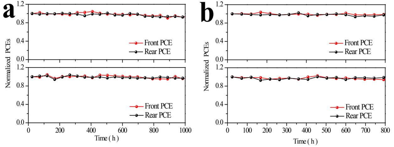
**Fig.S11** Normalized PCEs of bifacial CsPbBr<sub>3</sub> solar cells without QDs (above) and modified by CQDs/C-ZQDs (below) at (a) 60% RH/25 °C and (b) 80°C/0% RH. All the devices are measured without encapsulation.
