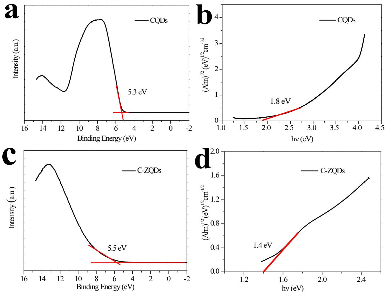
**Fig. S9** (a) High-resolution UPS analysis and b)  $(Ah\nu)^2$  vs energy ( $h\nu$ ) curve for CQDs. (c) High-resolution UPS analysis and (d)  $(Ah\nu)^2$  vs energy ( $h\nu$ ) curve for C-ZQDs.
