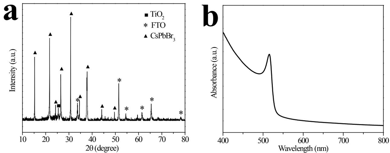
**Fig. S2** (a) XRD pattern of FTO/ $\text{TiO}_2$ / $\text{CsPbBr}_3$  configuration. (b) Typical UV-vis absorption spectrum of all-inorganic  $\text{CsPbBr}_3$  layer.
