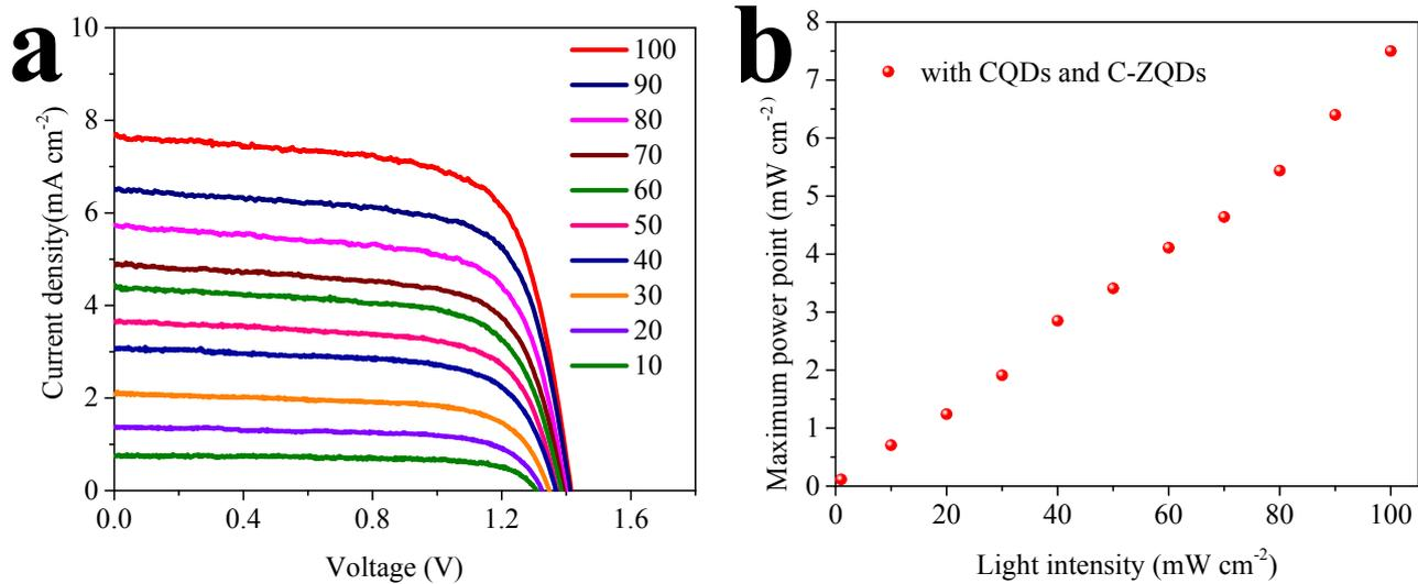
**Fig. S5** (a) The  $J$ - $V$  curves of CQDs/C-ZQDs modified PSC under front illumination with simulated sunlight intensity from 10 to 100 mW cm<sup>-2</sup>. (b) The plots of front  $P_{\max}$  as a function of  $P_{\text{in}}$ .
