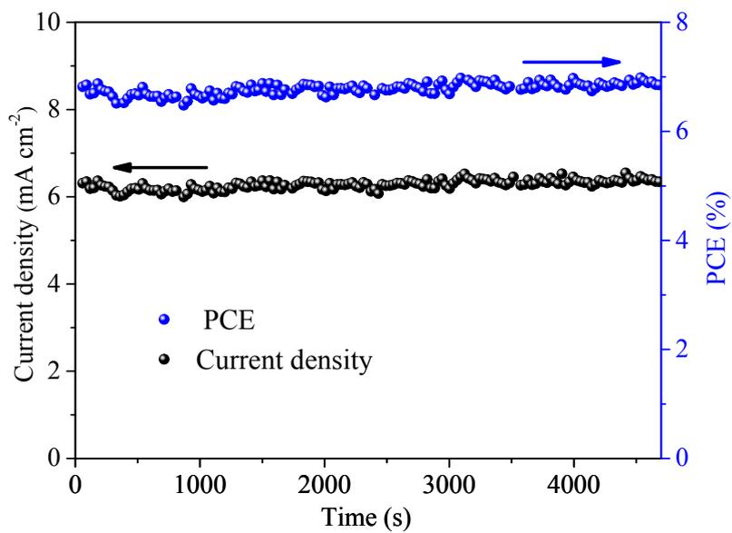
**Fig. S13** The continuous photocurrent density (left ordinate) and PCE (right ordinate) for CQDs/C-ZQDs modified bifacial PSCs under 1-sun light soaking.
