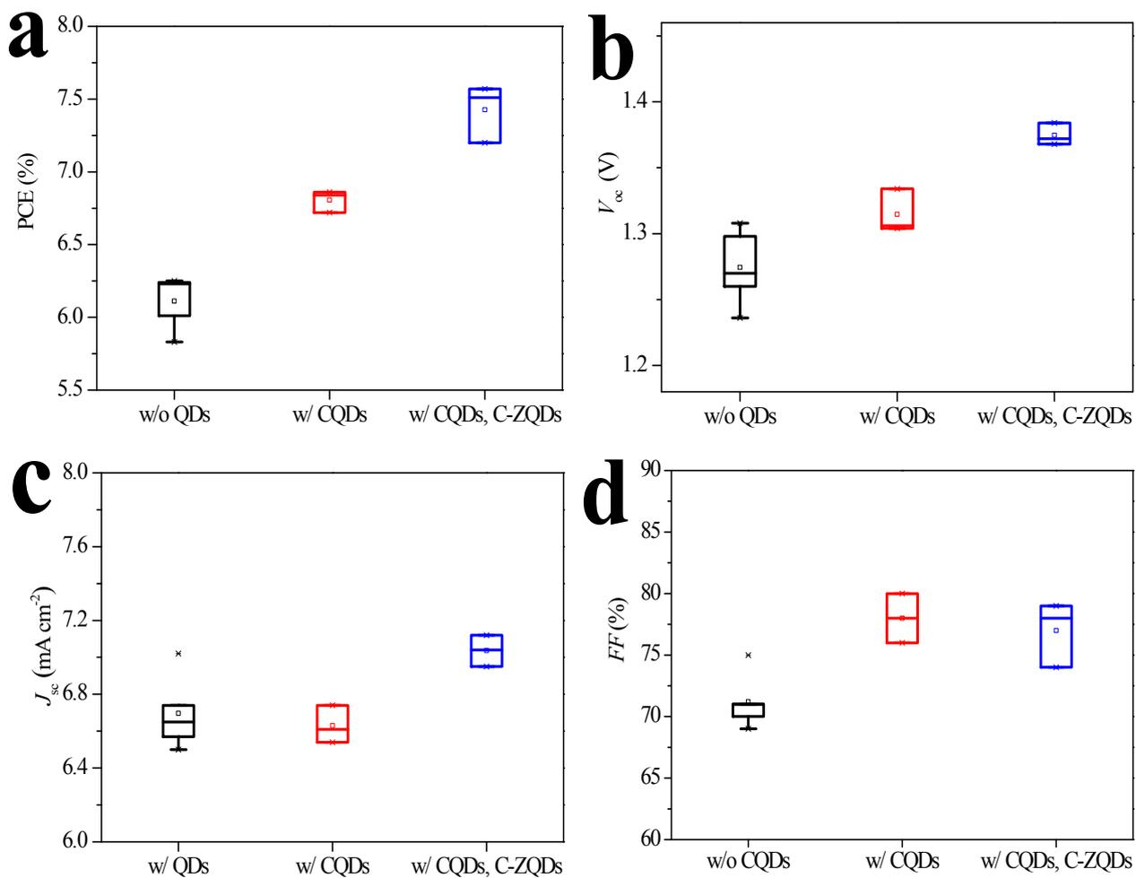
**Fig. S7** The statistical distribution of front photovoltaic parameters for three bifacial PSCs: (a) PCE, (b)  $V_{oc}$ , (c)  $J_{sc}$  and (d)  $FF$ .
