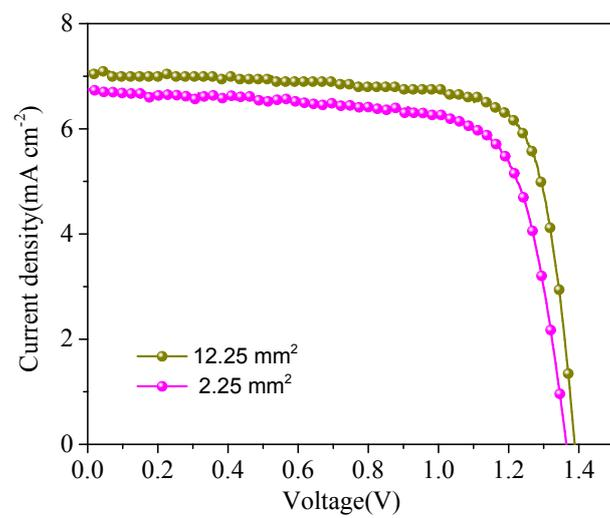
**Fig. S6** The  $J$ - $V$  curves of solar cells with different area (upon irradiation from front side).
