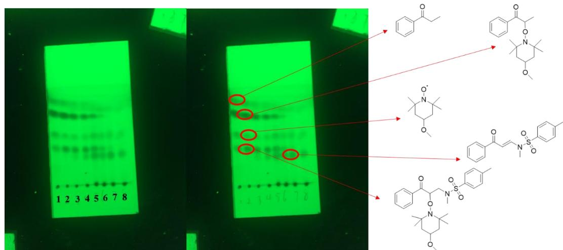
Collecting different samples from the same system at different reaction time (1-0.5h, 2-1h, 3-2h, 4-3h, 5-5h, 6-7h, 7-12h, 8-18h)
