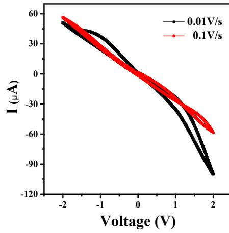
**Figure S4.** Working curves of the synaptic device under different scan rates.
