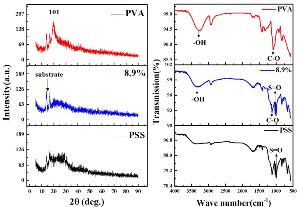
**Figure S2.** (a) XRD spectra of pure PVA, pure PSS and PSS hybrid PVA film. (b) Infrared spectroscopy of pure PVA, pure PSS and PSS hybrid PVA film.
