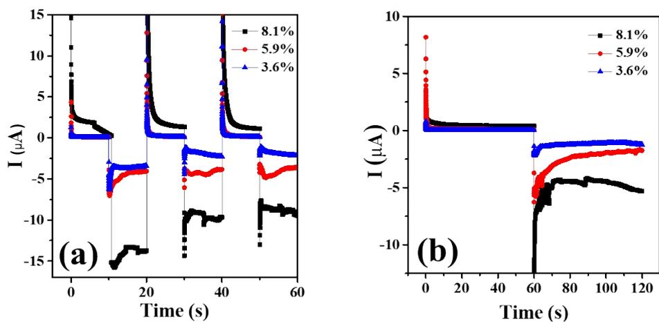
**Figure S3.** (a) Current responses of three diodes containing different PSS under AC field of 50 mHz with time. The repetitive biases applied are +2 V and -2 V. (b) Time dependence of current from diodes at constant forward (+2 V) and backward (-2 V) bias for long time.
