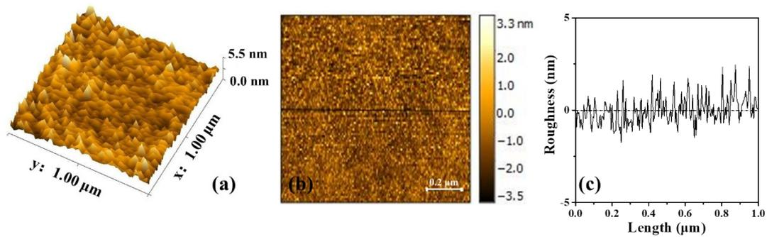
**Figure S1.** (a) and (b) AFM height image of the PSS hybrid PVA film. (c) AFM line scan of the film in (b).
