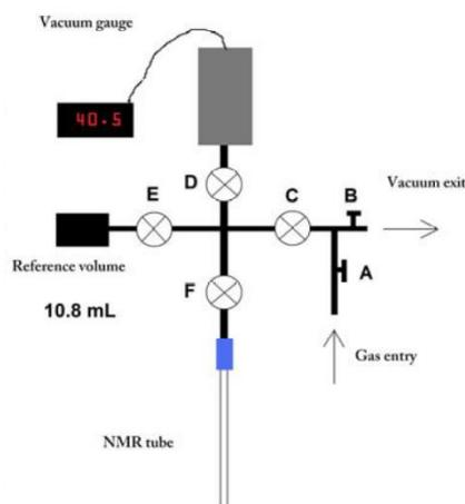
Figure S9. Schematic diagram of the system used for controlled loading of gases
