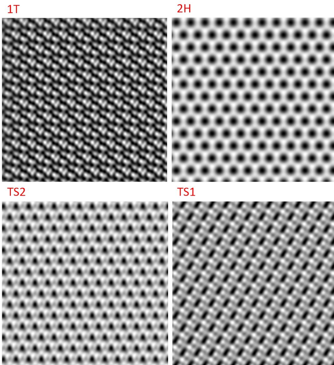
**Figure S9. TEM image simulation based on atomic model of single layer MoS<sub>2</sub> (Ovito Software) of different phases.**
