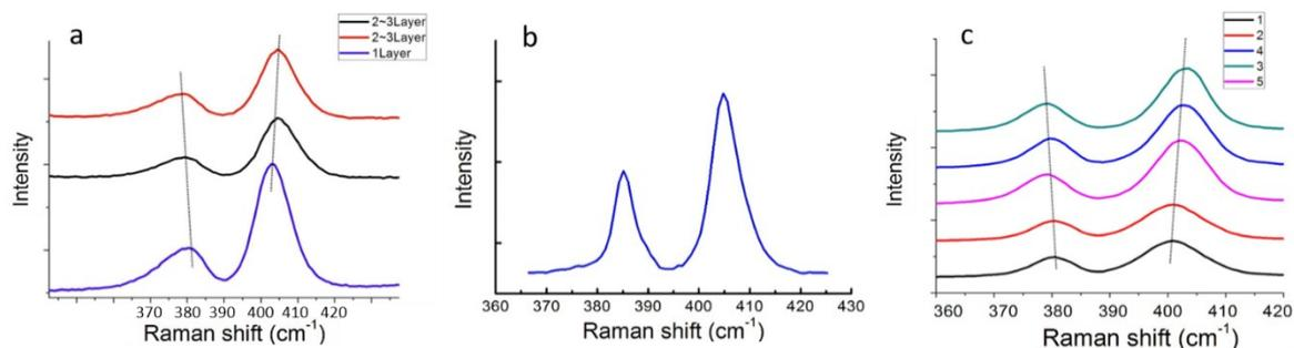
**Figure S3. Raman spectroscopy measurement.** (a) Raman shift correspond to the Figure 1(a)(b), which shows  $\Delta=20\text{cm}^{-1}\sim$ monolayer. (b) Raman shift correspond to the Figure 1(d), showing the layer composed of monolayer to trilayer. (c) Raman-shift of the netted-film layered, which shows a multilayer result.
