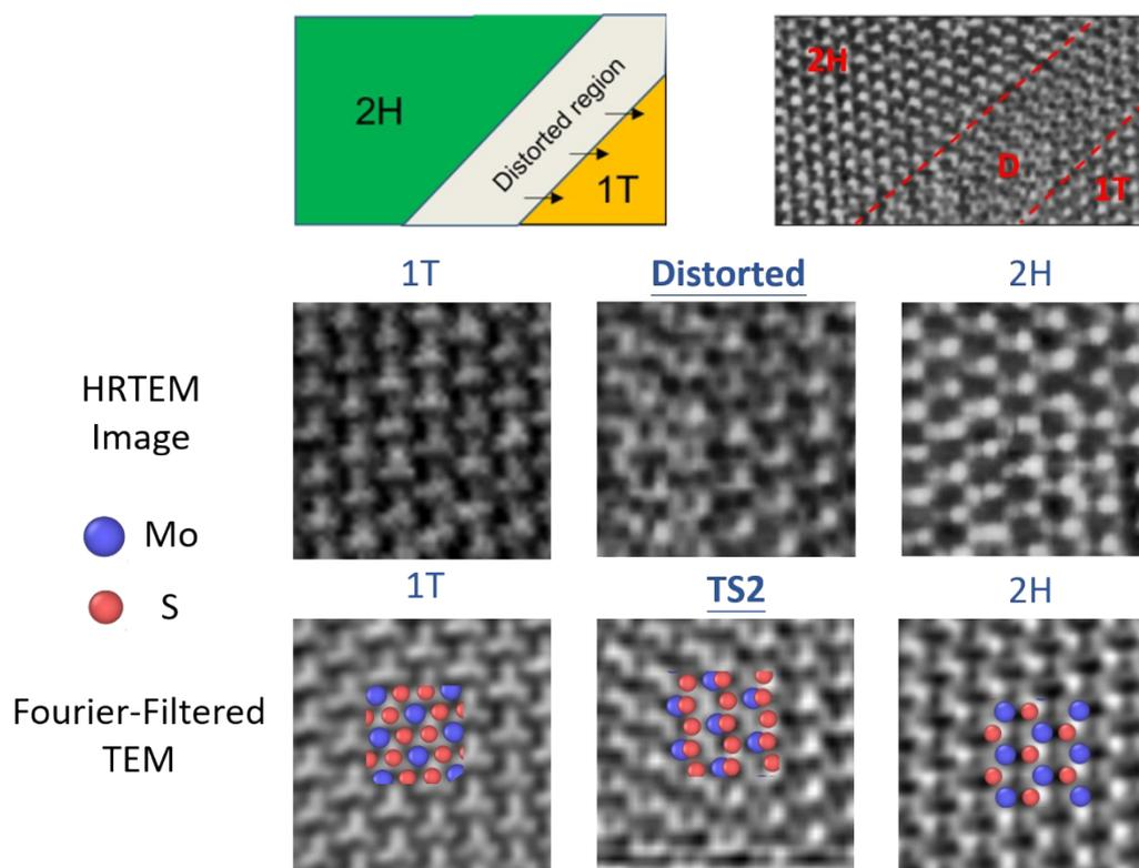
**Figure S7. The comparison between the established model and the experimental evidence.** The experimental image of 1T phase, the distorted region dragged out from figure 4c, and 2H phase. The Fourier-Filtered image were compared with the atomic model from figure S6.
