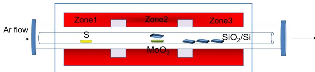
**Figure S1. Schematic illustration of the CVD system setting.**
