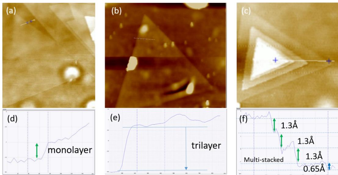
**Figure S2. AFM image and height profile** (a,d) AFM image shows the stacking layered MoS<sub>2</sub> and the height variation is 0.65nm (monolayer). (b,e) Another trilayer-growth MoS<sub>2</sub> with triangular domain and the height variation is 2.1nm(trilayer). (c) Multi-stacked pyramid MoS<sub>2</sub> was depicted in the AFM image. (f) Step height profile along the line indicated in (c).
