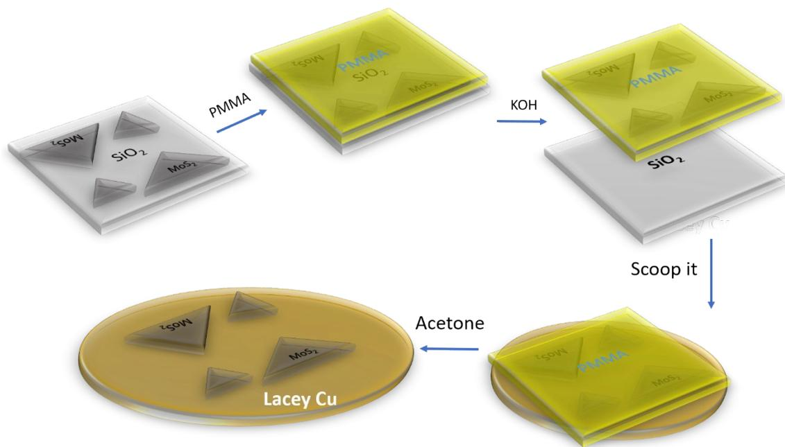
Figure S4. Illustration of transferring method.
