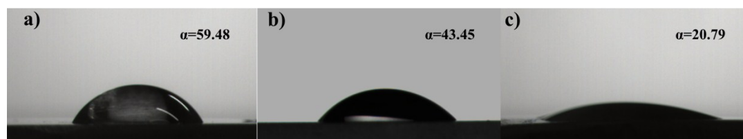
Fig. S3. Water contact angles of different titanium samples, uncoated surface (a), unmodified MP-KE coated surface (b), and modified MP-KE coated surface (c).
