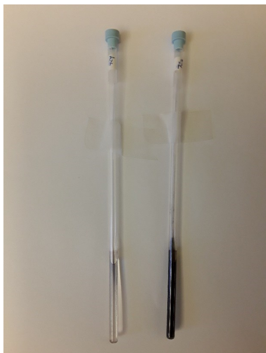
Figure S 3. Photographs of the NMR tubes after 24 hours of catalysis visually illustrating the different degree of decomposition when using 1 (left tube) and A (right tube) as a (pre)catalyst for the acetylene trifluoroacetylation.
