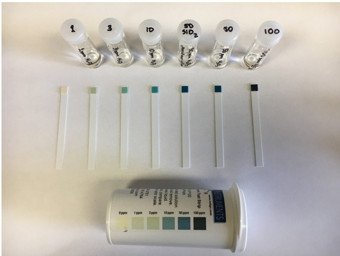
Figure S4. A visual “calibration curve” of known \text{H}_2\text{O}_2 concentrations. From left to right, a dry (not dipped) test strip, a strip dipped into a 1 ppm \text{H}_2\text{O}_2 solution, a strip dipped into a 3 ppm \text{H}_2\text{O}_2 solution, a strip dipped into a 10 ppm \text{H}_2\text{O}_2 solution, a strip dipped into a 50 ppm \text{H}_2\text{O}_2 solution that was passed through a silica plug in a pasteur pipette, a strip dipped into a 50 ppm \text{H}_2\text{O}_2 solution, and a strip dipped into a 100 ppm \text{H}_2\text{O}_2 solution,
