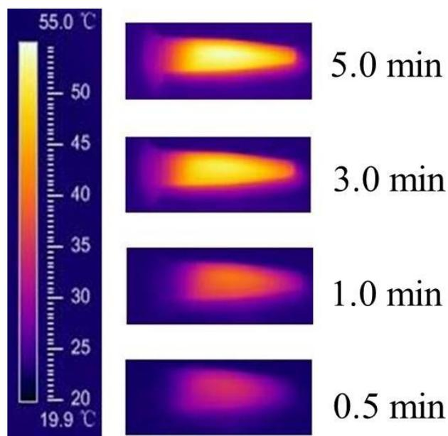
**Fig. S9** Infrared thermal images of the vesicles in water after laser irradiation for different times (660 nm, 1.5 W/cm<sup>2</sup>).
