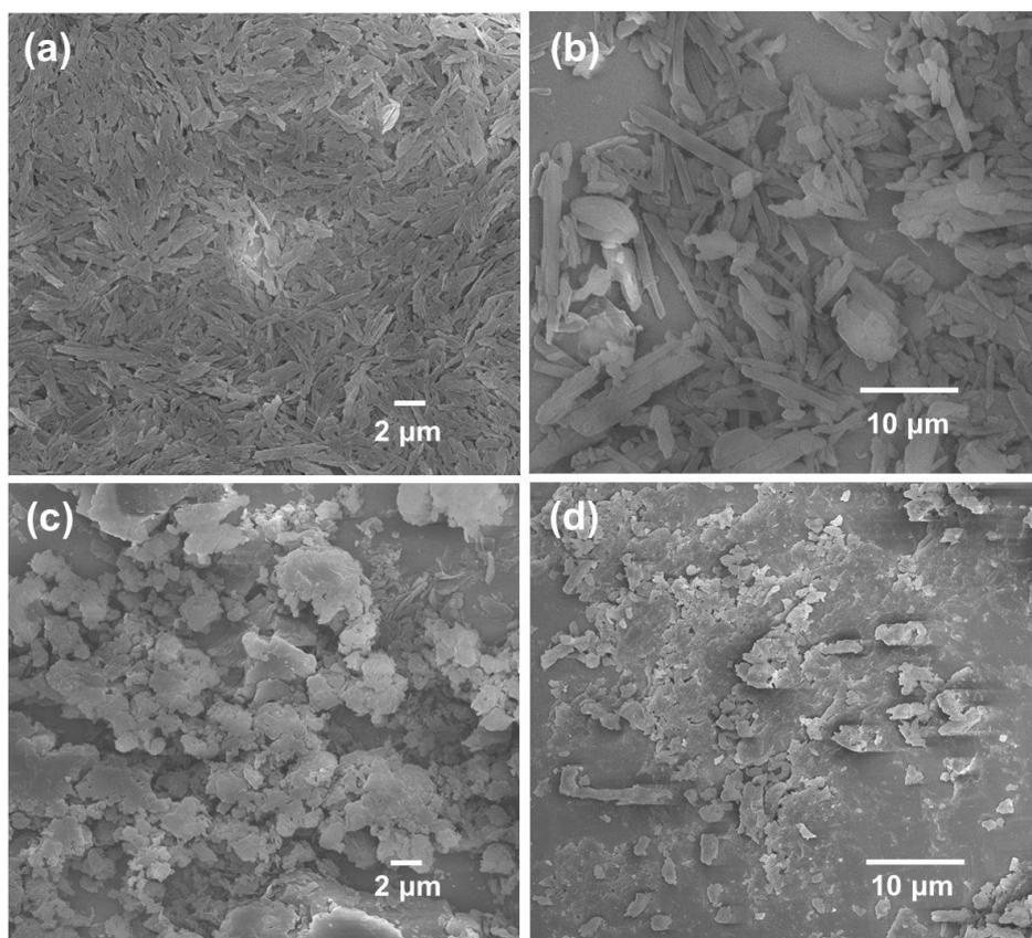
Fig. S3 SEM images of the pristine samples of (a) CPBT and (b) CTBT, and the ground samples of (c) CPBT and (d) CTBT.
