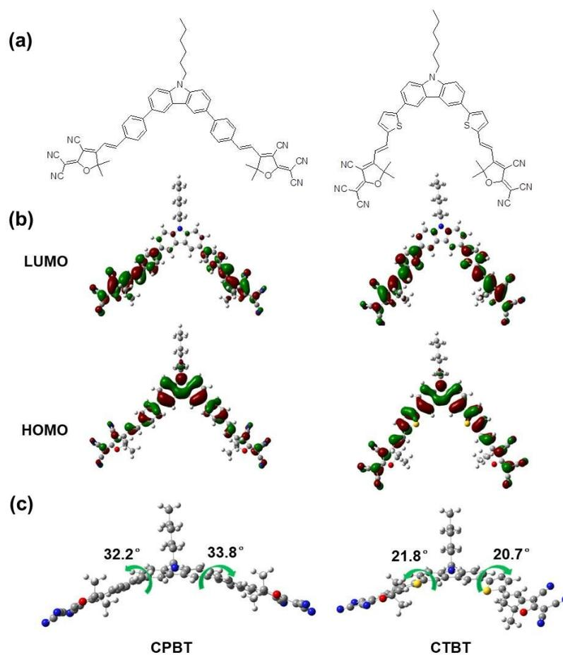
Fig. S1 (a) Molecular structure, (b) geometrically optimized HOMO and LUMO spatial distributions and (c) molecular conformations in THF solution of **CPBT** and **CTBT** obtained via DFT B3LYP/aug-cc-pVTZ calculations.
