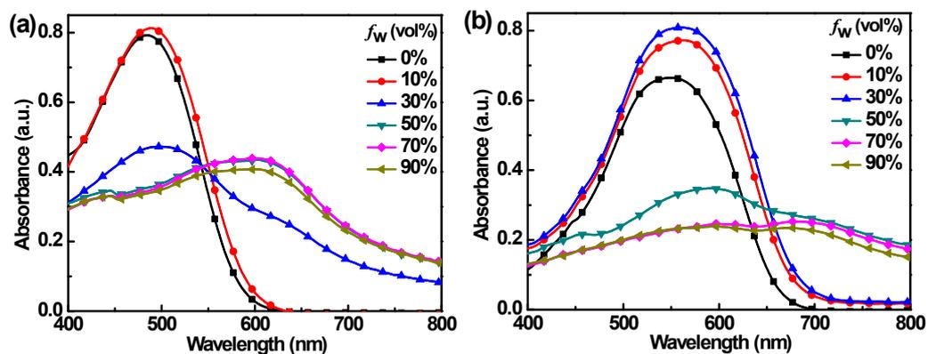
Fig. S2 UV-vis absorption spectra of (a) CPBT and (b) CTBT in THF/H<sub>2</sub>O mixtures with different water fractions ( $f_w$ s).
