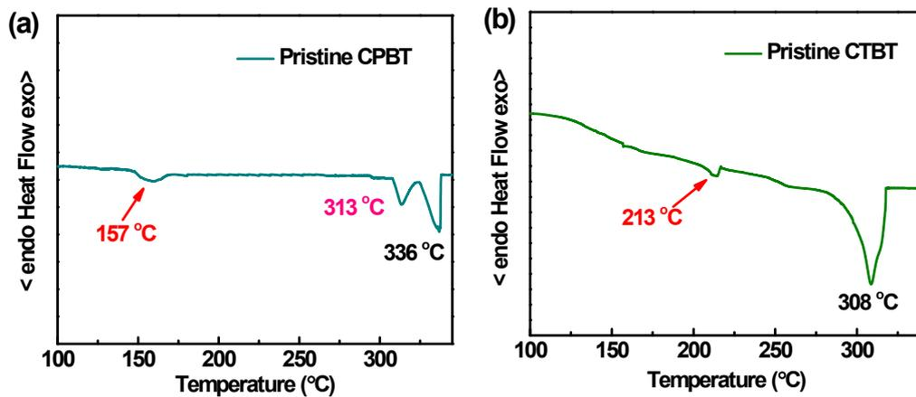
Fig. S4 DSC curves of the pristine samples of (a) CPBT and (b) CTBT.
