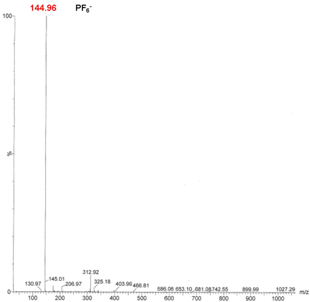
**Figure S31.** ESI-TOF (negative mode) mass spectrum of cofacial porphyrin dimer [Ag<sub>4</sub>(1)<sub>2</sub>](PF<sub>6</sub>)<sub>4</sub>.
