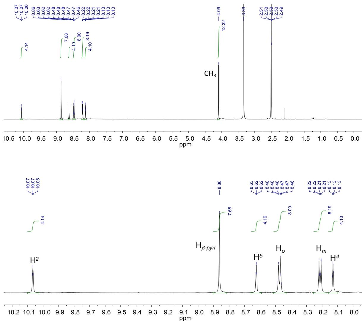
**Figure S11.** Full range (top) and partial (bottom) <sup>1</sup>H NMR spectra (600.3 MHz, DMSO-*d*<sub>6</sub>, 298 K) of porphyrin 4.
