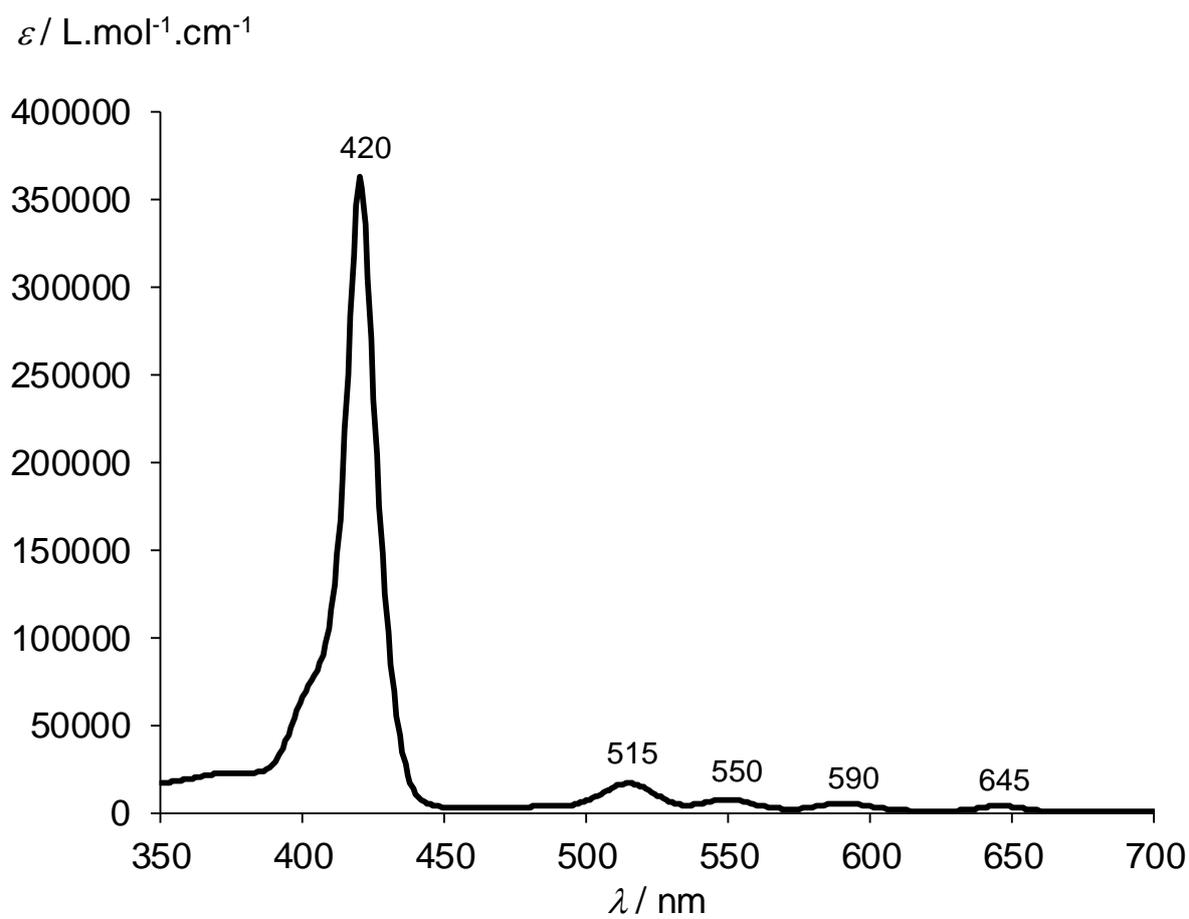
**Figure S3.** UV-vis spectrum (DMSO) of porphyrin **3I**.
