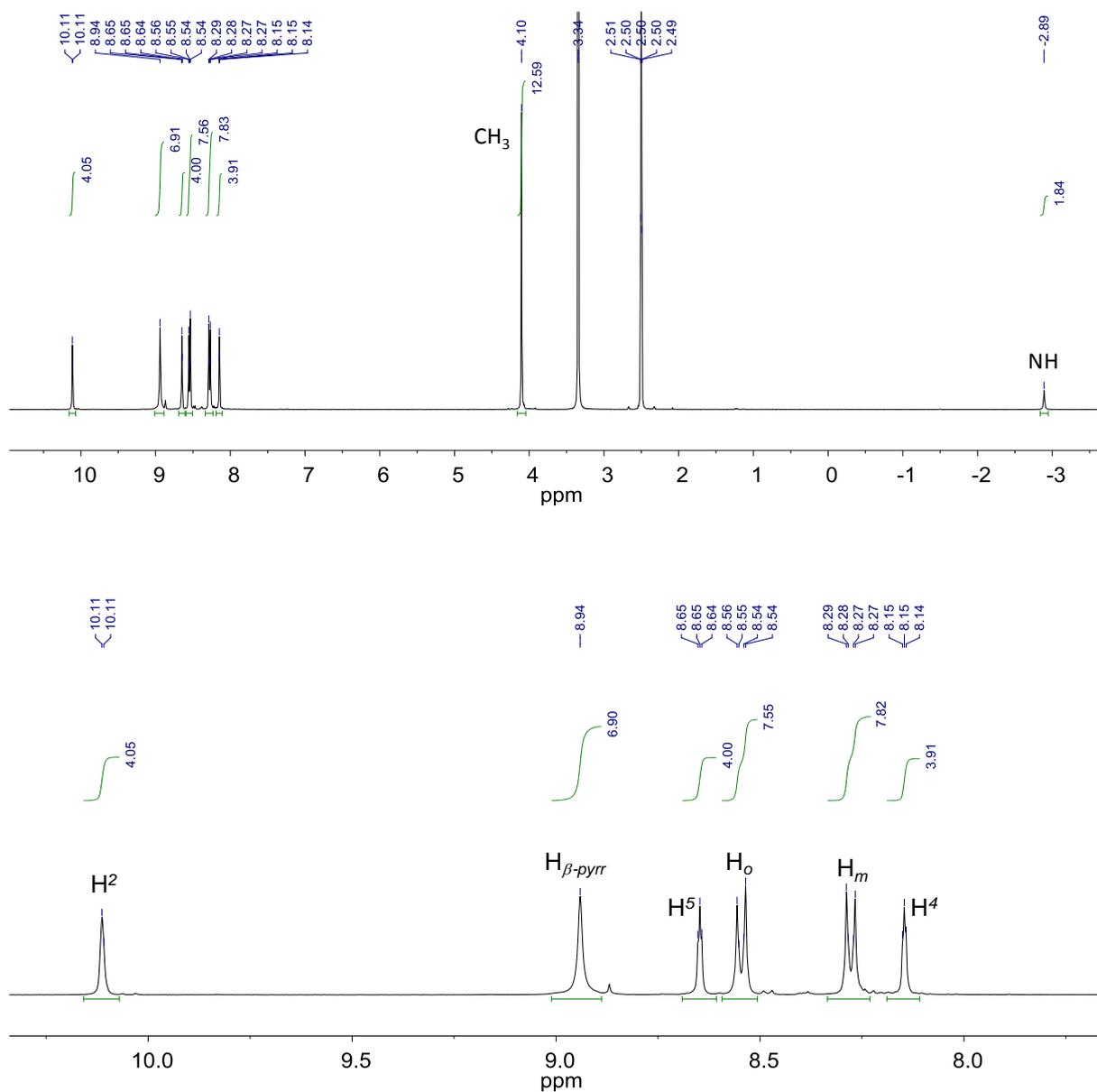
**Figure S1.** Full range (top) and partial (bottom) <sup>1</sup>H NMR spectra (400.1 MHz, DMSO-*d*<sub>6</sub>, 298 K) of porphyrin 3I.
