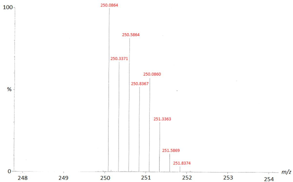
**Figure S20.** High-resolution ESI-TOF (positive mode) mass spectrum of porphyrin 4.
