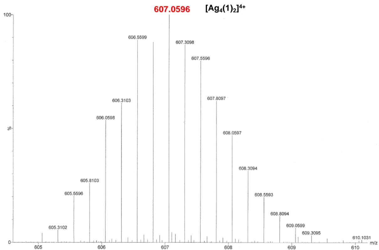
**Figure S30.** High resolution ESI-TOF (positive mode) mass spectrum of cofacial porphyrin dimer  $[\text{Ag}_4(\mathbf{1})_2](\text{PF}_6)_4$ .
