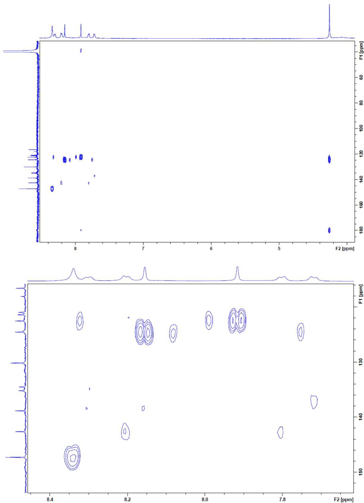
**Figure S28.** Full range (top) and partial (bottom)  $^1\text{H}$ - $^{13}\text{C}$  HMBC NMR spectra (600.3 MHz,  $\text{DMSO-}d_6$ , 298 K) of cofacial porphyrin dimer  $[\text{Ag}_4(\mathbf{1})_2](\text{PF}_6)_4$ .
