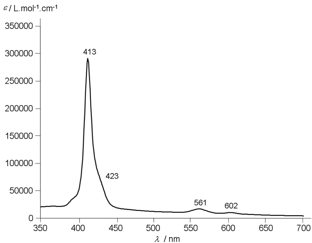
**Figure S29.** UV-vis spectrum (DMSO) of cofacial porphyrin dimer  $[\text{Ag}_4(\mathbf{1})_2](\text{PF}_6)_4$ .
