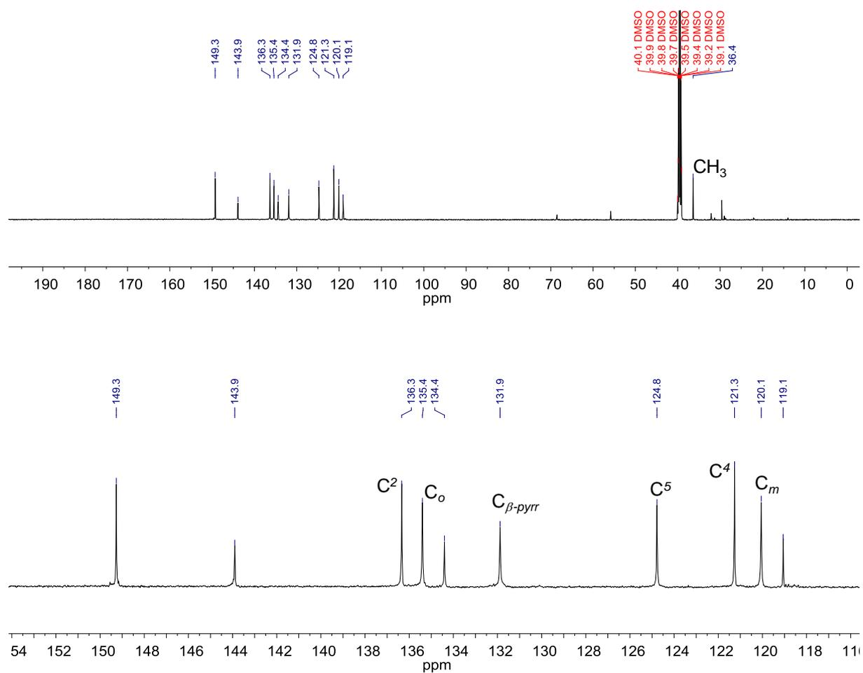
**Figure S16.** Full range (top) and partial (bottom)  $^{13}\text{C}\{^1\text{H}\}$  NMR spectra (150.9 MHz,  $\text{DMSO-}d_6$ , 298 K) of porphyrin **4**.
