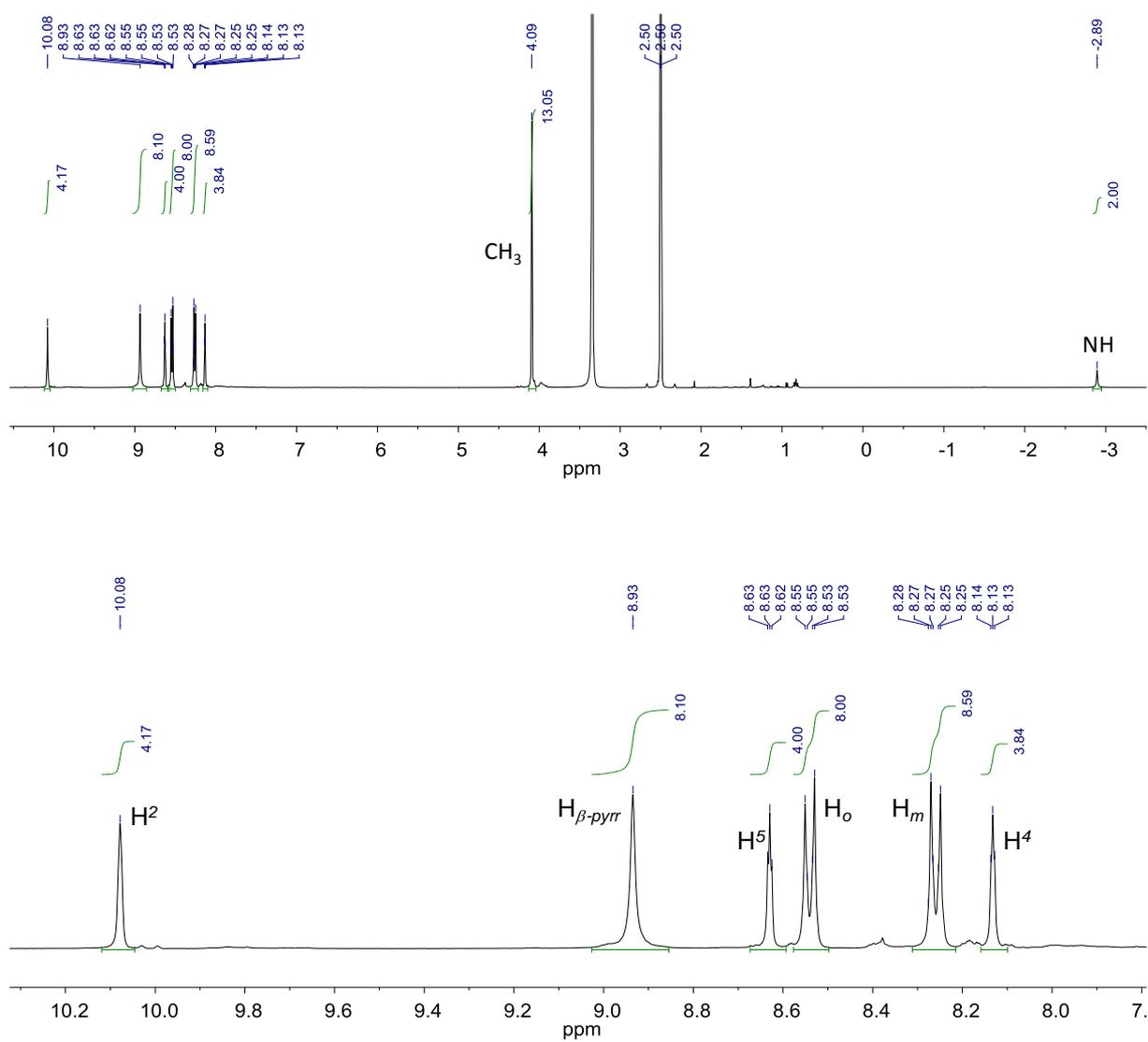
**Figure S5.** Full range (top) and partial (bottom) <sup>1</sup>H NMR spectra (400.1 MHz, DMSO-*d*<sub>6</sub>, 298 K) of porphyrin 3PF<sub>6</sub>.
