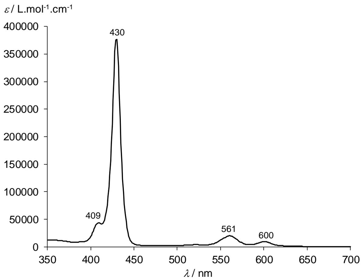
**Figure S18.** UV-vis spectrum (DMSO) of porphyrin 4.
