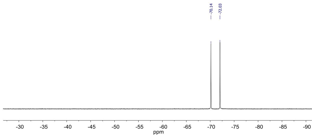
**Figure S25.**  $^{19}\text{F}$  NMR spectra (376.5 MHz,  $\text{DMSO-}d_6$ , 298K) of cofacial porphyrin dimer  $[\text{Ag}_4(\mathbf{1})_2](\text{PF}_6)_4$ .
