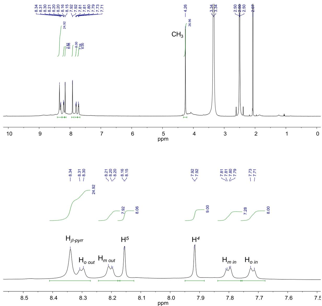
**Figure S21.** Full range (top) and partial (bottom)  $^1\text{H}$  NMR spectra (600.3 MHz,  $\text{DMSO-}d_6$ , 298 K) of cofacial porphyrin dimer  $[\text{Ag}_4(\mathbf{1})_2](\text{PF}_6)_4$ .
