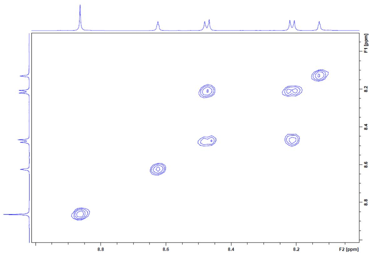
**Figure S12.**  $^1\text{H}$ - $^1\text{H}$  COSY NMR spectrum (600.3 MHz,  $\text{DMSO-}d_6$ , 298 K) of porphyrin **4**.
