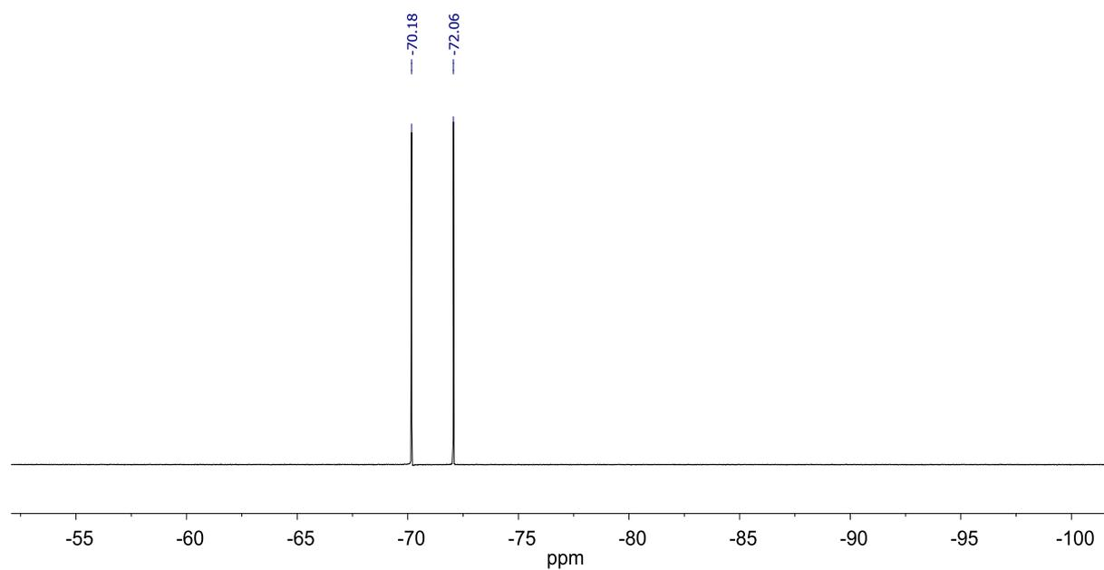
**Figure S15.**  $^{19}\text{F}$  NMR spectrum (376.5 MHz,  $\text{DMSO-}d_6$ , 298 K) of porphyrin **4**.
