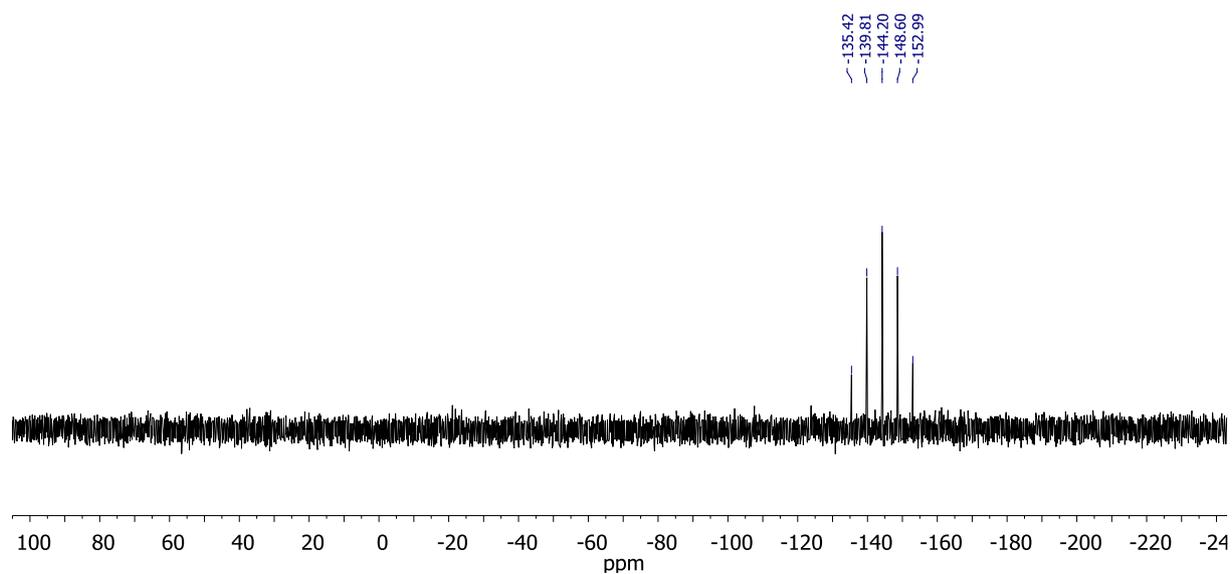
**Figure S14.**  $^{31}\text{P}$  NMR spectrum (162 MHz,  $\text{DMSO-}d_6$ , 298 K) of porphyrin **4**.
