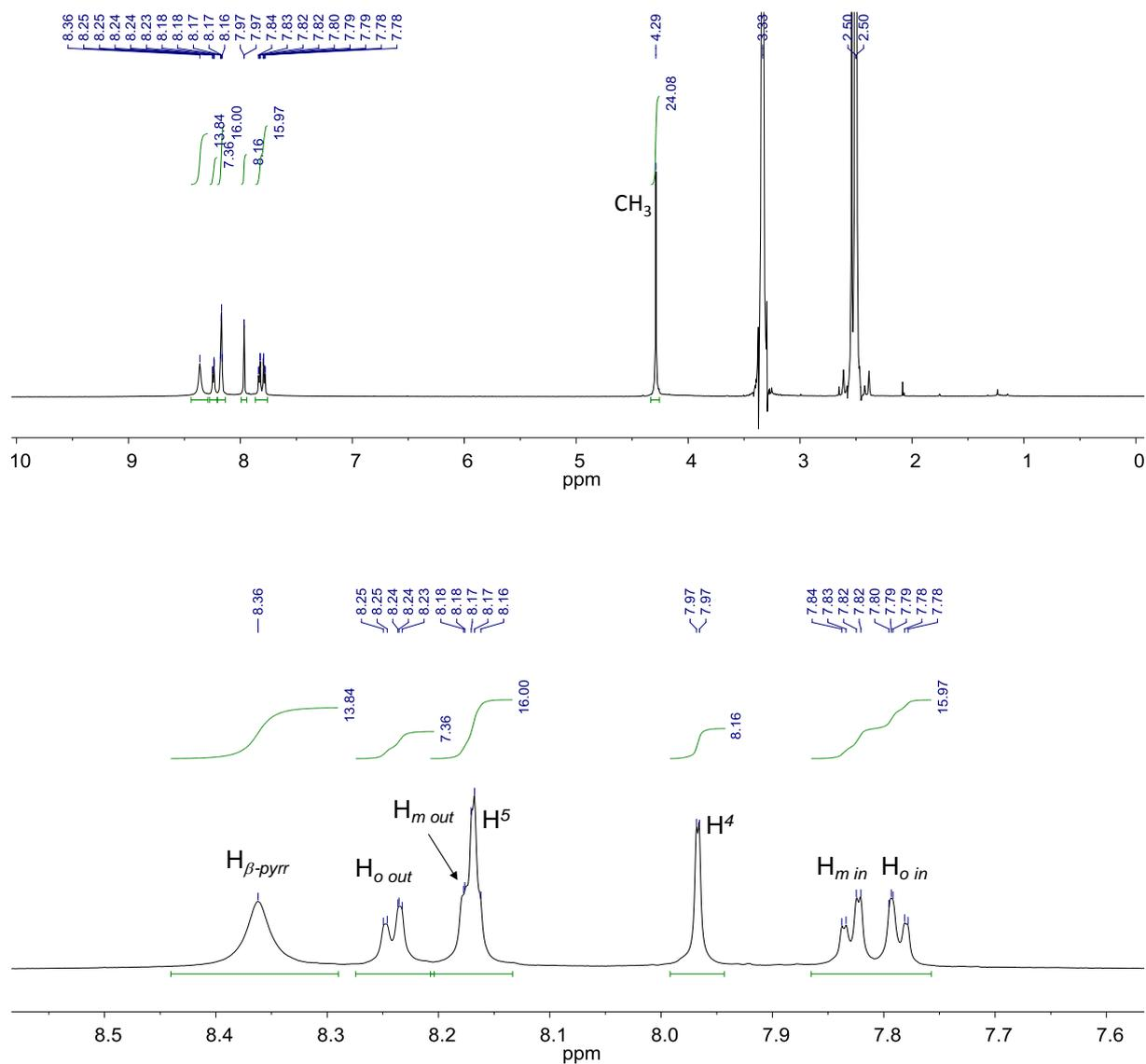
**Figure S32.** Full range (top) and partial (bottom) <sup>1</sup>H NMR spectra (600.3 MHz, DMSO-*d*<sub>6</sub>, 298 K) of cofacial porphyrin dimer [Au<sub>4</sub>(1)<sub>2</sub>](PF<sub>6</sub>)<sub>4</sub>.
