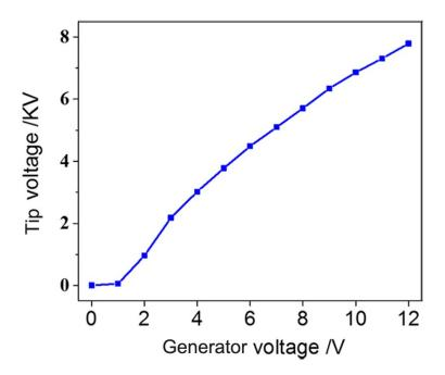
Figure S2 Characterization of the tungsten-tip voltage (absolute voltage) versus the output voltage from NAIs generator.
