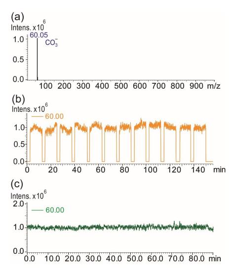
**Figure S3** (a) MS spectrum in the range of 10 to 1000 (m/z ratio) to characterize NAIs under the optimized parameters. (b) Reproducibility and (b) Long-time stability of NAIs. Output voltage of 5 V, synthetic air flow rate of 5 L/min, L of 3 mm, and D of 8 mm.
