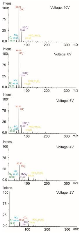
**Figure S1** MS characterization of untreated laboratory air. Output voltage of 12 V, L of 3 mm, and D of 8 mm.
