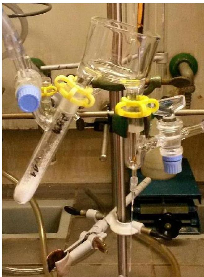
Figure S 3: Picture of the glass trousers and the capillary station for the transfer of the sample from the Schlenk apparatus to the capillary.
