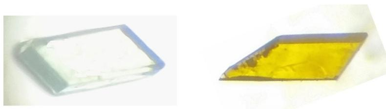
**Fig. S2** The photograph of compound **1** before and after ion exchange in 15 ml,  $1 \times 10^{-3} \text{ mol L}^{-1} \text{ K}_2\text{Cr}_2\text{O}_7$  solution. The adsorption process reached the dynamic balance state.
