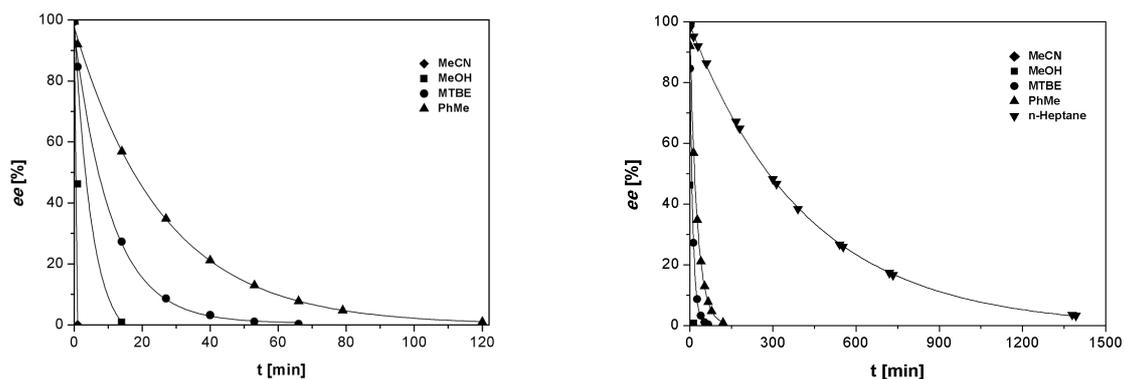
**Figure S1.** Racemization of **7a** (0.7 mg/mL) in the presence of DBU (3.3  $\mu$ L/mL) in different solvents excluding (*left*) and including (*right*) n-Heptane.
