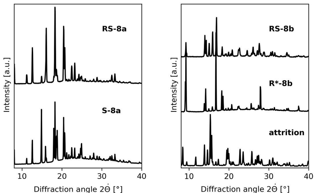
**Figure S7.** XRPD patterns of the identified conglomerates: **8a** (*RS* vs *S*; left) and **8b** (*RS* vs *R\** (absolute configuration was not confirmed) vs deracemization attempt; right).
