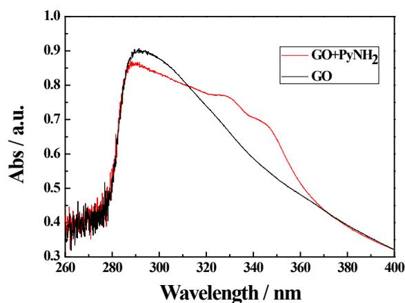
**Figure S1.** The UV-Vis absorption spectra of GO and GO loaded with PyNH<sub>2</sub> (GO+PyNH<sub>2</sub>).
