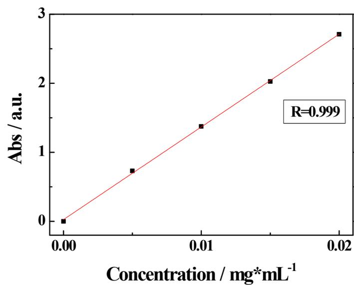
**Figure S2.** The absorbance standard curve line of PyNH<sub>2</sub>.
