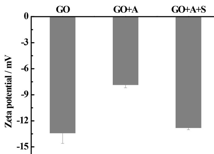
**Figure S3.** Zeta potential of GO, GO loaded with DR4 antibody (GO+A) and GO loaded with DR4 antibody and AKT siRNA (GO+A+S).
