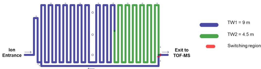
**Figure S1.** Diagram of SLIM SUPER module used in all experiments.
