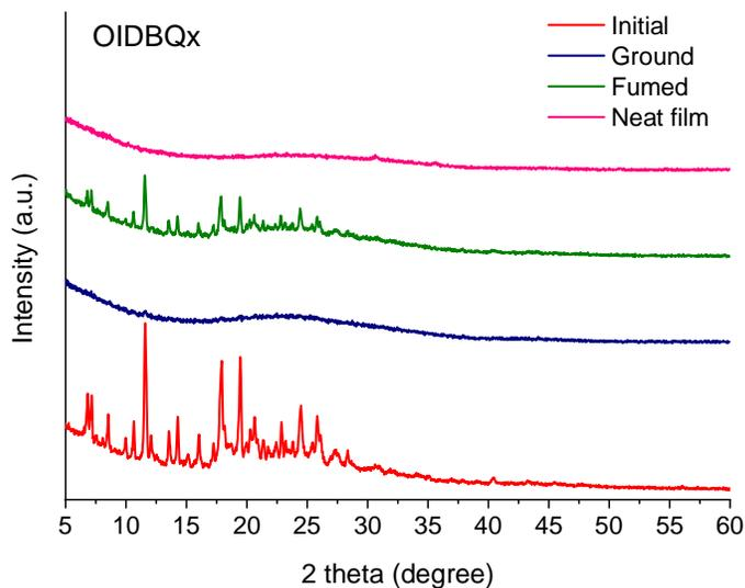
**Figure S16.** Powder Xray diffractogram of OIBDQx under application in initial form (-i), ground (-g), drop-cast film (-df) and after fumigation (-f).
