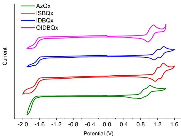
**Figure S5.** Oxidation and reduction potential of compounds in DCM recorded with cyclic voltammetry.
