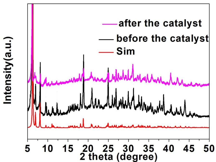
**Fig. S5** The PXRD pattern of recycled samples before the catalyst and after catalyst.
