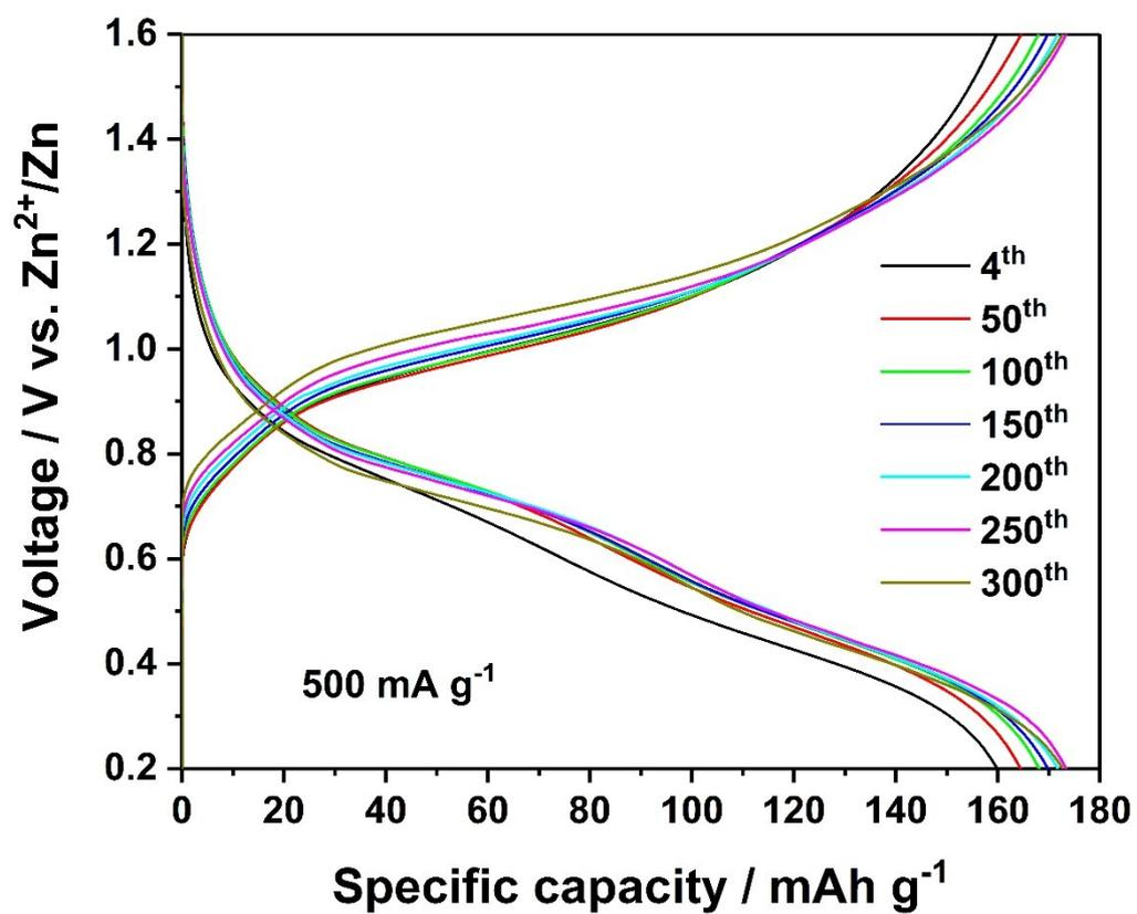
Figure S4. Selected voltage profiles at 500 mA g<sup>-1</sup> of CVO electrode.
