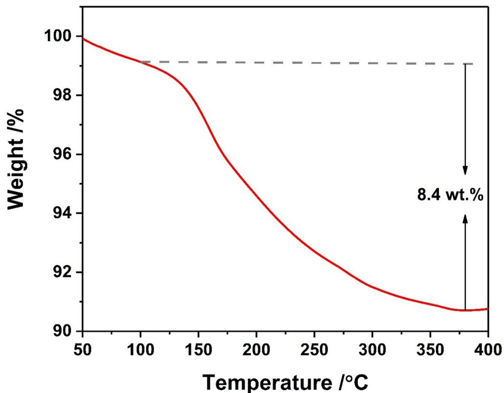
Figure S2. TGA curve of as-prepared CVO.
