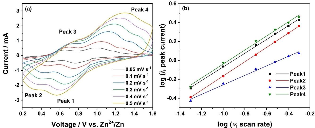
Figure S3. (a) CV curves of CVO at different scan rates of 0.05, 0.1, 0.2, 0.3, 0.4, 0.5 mV s<sup>-1</sup>.
