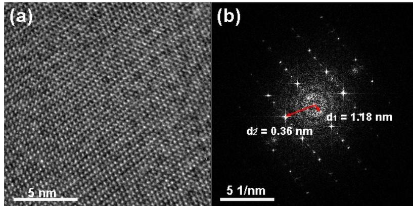
Figure S6. (a) HRTEM of fully discharged CVO, and (b) corresponding FFT image (diffraction pattern).
