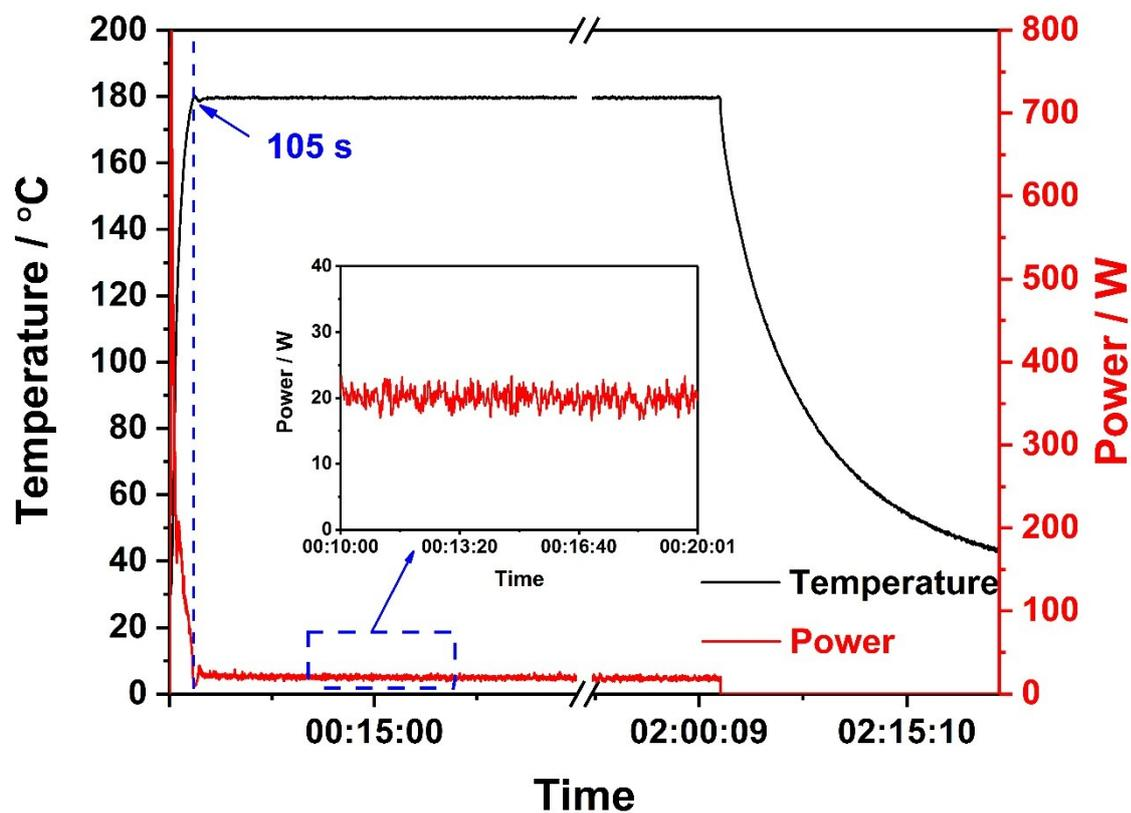
Figure S1. Evolution of temperature and power during the microwave reaction. The data was directly recorded by the microwave oven. The inset shows the power needed to keep the temperature constant from 10 to 20 min.
