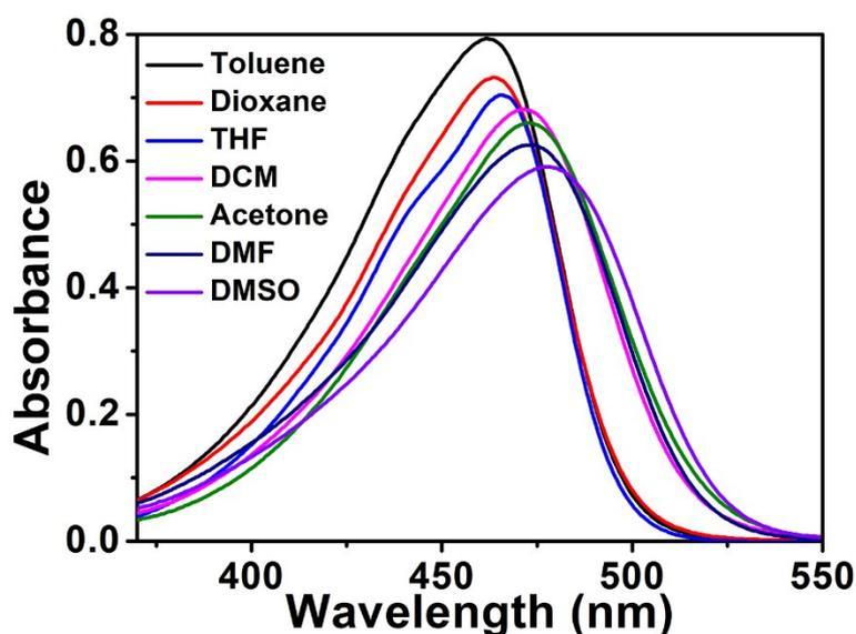
Fig. S1. The absorption spectra of CTPA in different polarity solvents.
