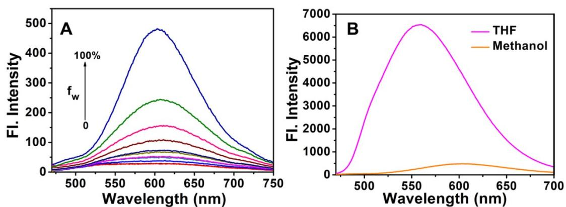
**Fig. S6.** (A) The fluorescence spectra of CTPA (10  $\mu$ M) under different viscosity in methanol-glycerol system with the fraction of glycerol ( $f_w$ ) from 0 to 100%. (B) The fluorescence spectra of CTPA in THF and methanol. THF and methanol have almost the same viscosity (0.53 cP vs 0.60 cP) but different polarity ( $E_T(30) = 37.4$  vs 55.4)
