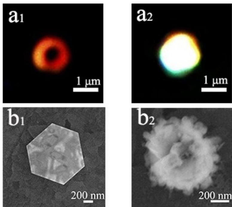
**Figure S12.** (a1, b1) DFM images of AuHNPs before and after their interaction with  $\text{Hg}^0$ . (a2, b2) SEM images of the same nanoplate. The edge effect disappears and strong white light spot appears subsequently after direct exposure of AuHNPs to liquid  $\text{Hg}^0$  generated by reducing  $\text{Hg}^{2+}$  with ascorbic acid.
