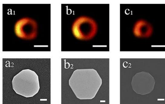
**Figure S9.** DFM images of irregular Au nanoplates (a1-c1, scale bar is 1  $\mu\text{m}$ ) and their corresponding SEM images (a2-c2, scale bar is 300 nm). Different shapes of nanoplates also show similar edge effect if the size is beyond diffraction limit (about 200 nm).
