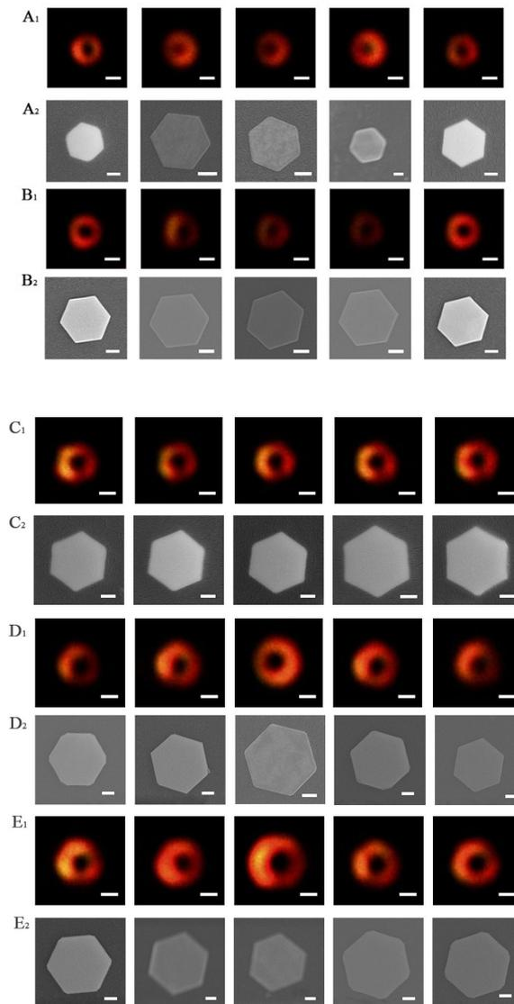
**Figure S4.** Doughnut-shaped far-field scattering patterns (DNSPs) of representative regular AuHNPs in the range of 500-1000 nm. (A1–E1) DFM images (the scale bar is 500 nm); (A2–E2) the corresponding SEM images (the scale bar is 200 nm). It can be seen that the DFM images exhibit similar DNSPs in spite of different sizes.
