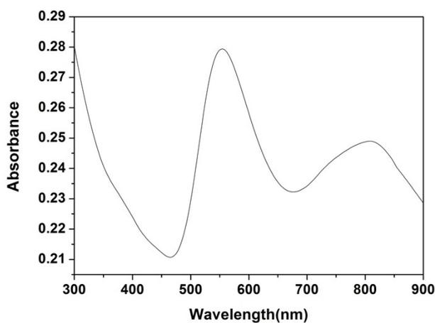
**Figure S2.** UV-Vis spectra of Au plate-like nanostructures and pseudospherical nanoparticles. The low- and high-energy peaks are attributed to the dipolar resonance of the pseudo-spherical nanoparticles and surface plasmon resonance modes of the AuHNPs that lie within the plane of the nanoplates, respectively.
