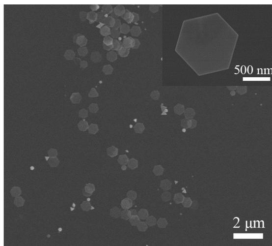
**Figure S1.** The SEM images of as-prepared gold regular hexagonal nanoplates (AuHNPs). The resulting AuHNPs solution through wet-chemical syntheses in organic media contains a mixture of plate-like nanostructures and pseudospherical nanoparticles. About 40% of the as-prepared AuHNPs are regular according to the statistics of the SEM images by accounting 100 particles.
