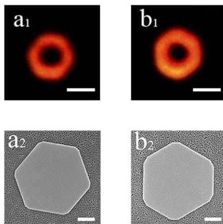
**Figure S8.** DFM images of AuHNPs larger than 1000 nm (a1-b1, scale bar is 1  $\mu\text{m}$ ) and their corresponding SEM images (a2-b2, scale bar is 300 nm). The shapes of scattering images present obvious hexagonal profile in DFM, whose orientations are in the agreement with authentic external contour obtained by SEM.
