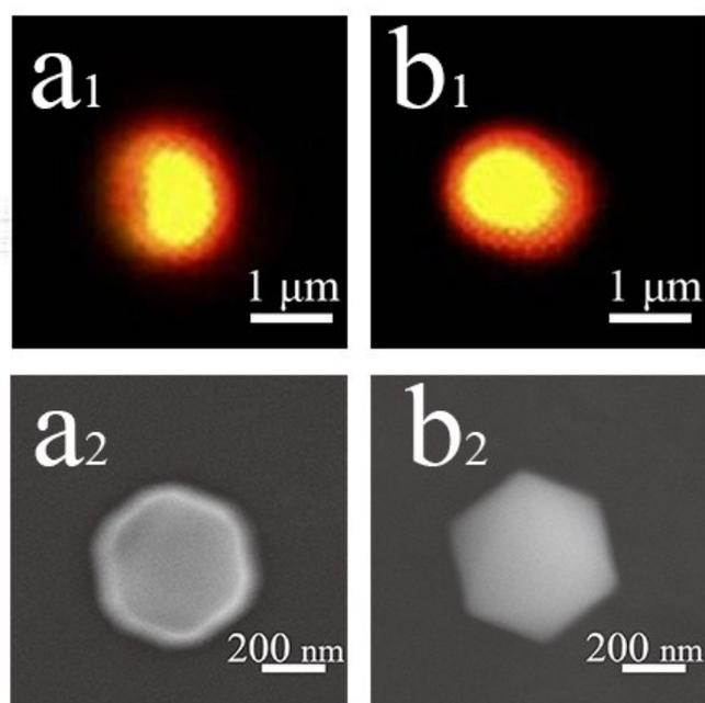
**Figure S3.** DFM image of AuHNPs smaller than 500 nm. (a1-b1) and their corresponding SEM images (a2-b2). The scattering images exhibit elongated solid bright spot.
