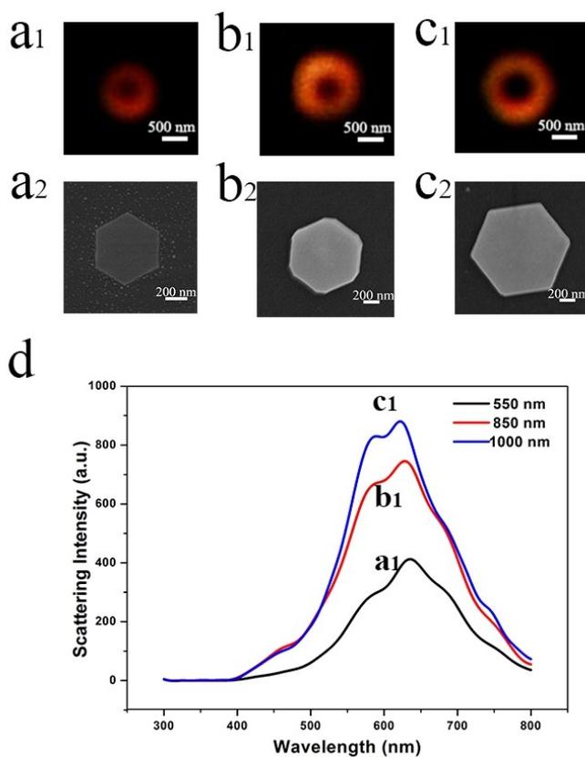
**Figure S7.** DFM images of AuHNPs with 550 nm, 850 nm, 1000 nm. (a1-c1), their SEM images (a2-c2), and their corresponding scattering spectra (d). Light scattering spectra of different sizes exhibited similar peak position but different scattering intensity. It can be concluded that the appearance of edge effect of different sizes is independent of scattering spectra.
