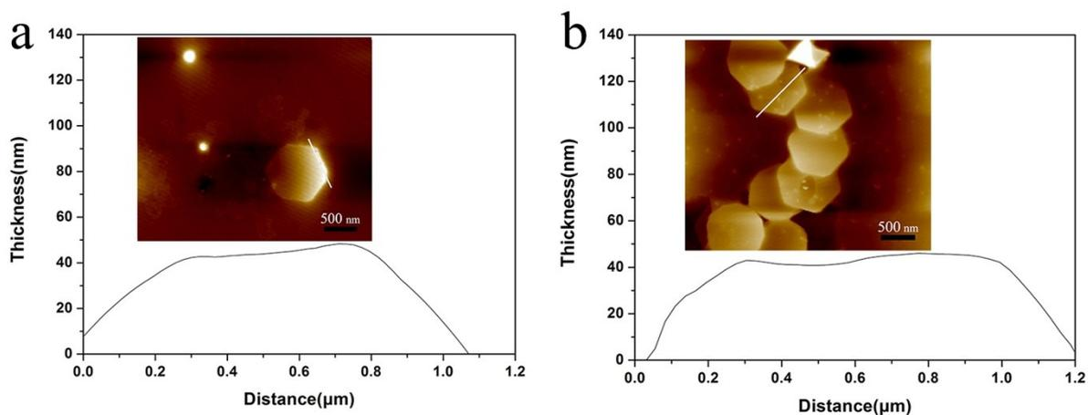
**Figure S6.** AFM images and height profiles of AuHNPs.
