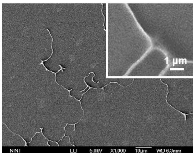
Figure S3: SEM image of MS before tyrosinase treatment
