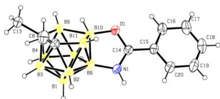
**Figure S4. Crystal structure of 3q.**
