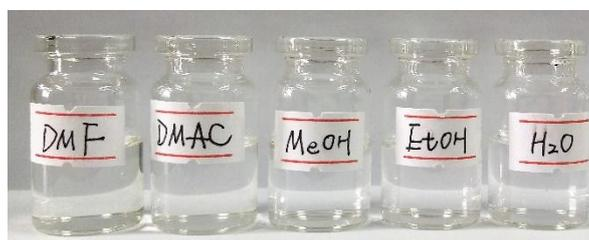
**Figure S4.** The filtrate of  $\text{Mo}_3\text{S}_{13}$ @EB-COF in different solvents after 24 hours soakage.
