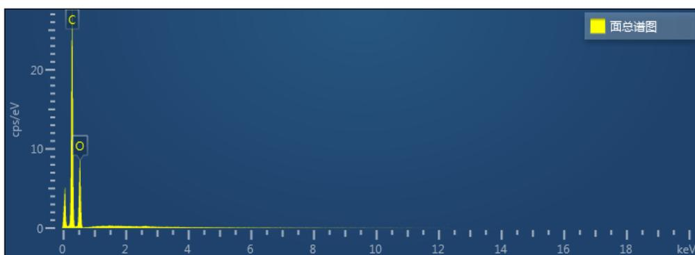
**Figure S20.** EDS elemental analysis of the filtrate after photocatalytic hydrogen evolution.
