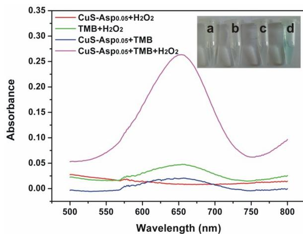
**Figure S4.** Different combinations of CuS-Asp<sub>0.05</sub>, H<sub>2</sub>O<sub>2</sub>, and TMB in 0.1 M PBS (pH 7.0). The inset shows the corresponding photograph (a—TMB+H<sub>2</sub>O<sub>2</sub>, b—CuS-Asp<sub>0.05</sub>+TMB, c—CuS-Asp<sub>0.05</sub>+H<sub>2</sub>O<sub>2</sub>, d—CuS-Asp<sub>0.05</sub>+H<sub>2</sub>O<sub>2</sub>+TMB).
