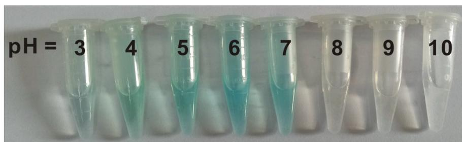
**Figure S16.** The TMB color reaction catalyzed by glutamic acid-modified CuS in buffers with different pH values.
