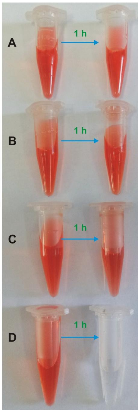
**Figure S7.** Degradation of Congo red in different systems (A—None, B—CuS-Asp<sub>0.05</sub>, C—H<sub>2</sub>O<sub>2</sub>, D—CuS-Asp<sub>0.05</sub>+H<sub>2</sub>O<sub>2</sub>).
