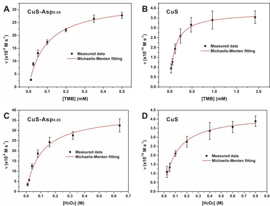
**Figure S14.** Steady-state kinetic measurements of (A and C) CuS-Asp<sub>0.05</sub> and (B and D) bare CuS toward (A and B) TMB and (C and D) H<sub>2</sub>O<sub>2</sub> in neutral media.
