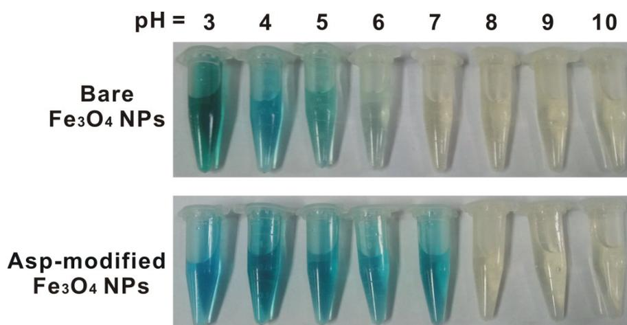
**Figure S18.** The TMB color reaction catalyzed by bare Fe<sub>3</sub>O<sub>4</sub> NPs and Asp-modified
