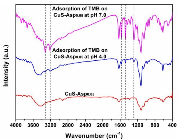
**Figure S17.** FT-IR spectra of CuS-Asp<sub>0.05</sub> before and after adsorption of TMB at different pH values. The absorption signals labeled with dashed line are attributed to the TMB substrate adsorbed on the nanozyme.
