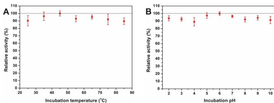
**Figure S9.** Robustness of the CuS-Asp<sub>0.05</sub> nanozyme against (A) harsh temperature and (B) pH.
