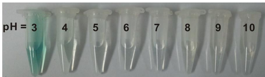
**Figure S15.** The ABTS color reaction catalyzed by CuS-Asp<sub>0.05</sub> in buffers with different pH values.
