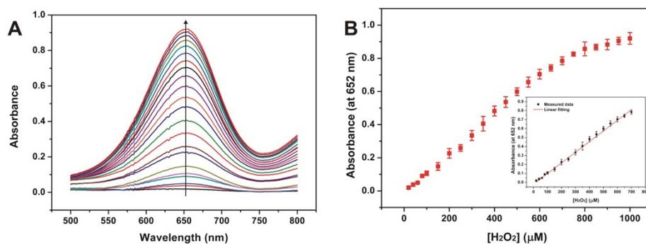
**Figure S19.** (A) displays the UV-Vis spectra of the CuS-Asp<sub>0.05</sub>+H<sub>2</sub>O<sub>2</sub>+TMB system with different concentrations of H<sub>2</sub>O<sub>2</sub>. (B) shows the relationship between the H<sub>2</sub>O<sub>2</sub> level and the absorbance at 652 nm.
