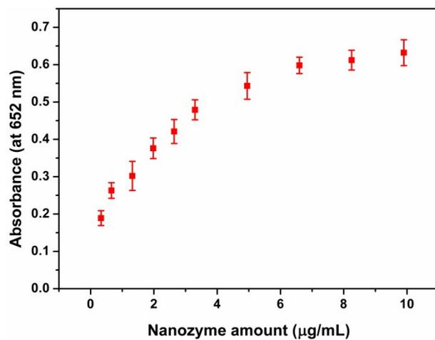
**Figure S12.** Effect of the CuS-Asp<sub>0.05</sub> amount used on the TMB color reaction.
