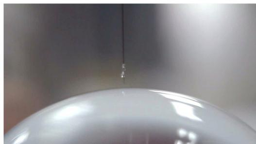
**Fig. S2** Cr electrodeposition was conducted in convex-shaped Sargent bath in order to obtain still surface (a). Water droplets appeared on the electrode tip when the bath temperature was 50°C (b). Experiment in (b) was conducted using water.
