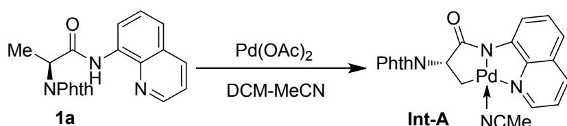
To an oven-dried 50 mL round-bottomed flask was added substrate **1a** (1.0 mmol), Pd(OAc)<sub>2</sub> (1.0 mmol) in DCM (10 mL) and MeCN (5 mL). The flask was stirred for 12 h at 60 °C followed by cooling. The purified product was collected by filtration, washed with MeCN, diethyl ether and dried under vacuum to afford **Int-A** (392 mg,
