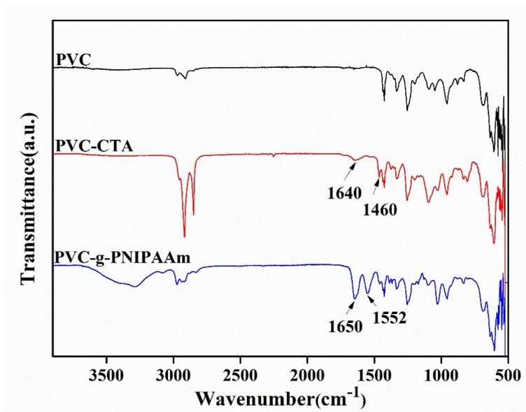
Figure S15. Reflectance FT-IR spectra of PVC, PVC-CTA and PVC-g-PNIPAAm surfaces.
