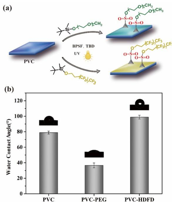
**Figure S18.** (a) One-step photoimmobilization of PEG or HDFD on PVC surfaces. (b) Sessile water drop contact angles of the unmodified PVC, PVC-PEG and PVC-HDFD substrates. The data are presented as the standard deviation ( $n = 6$ ).
