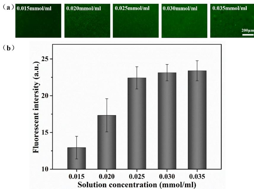
**Figure S20.** (a) Fluorescence microscopy images of the PVC-SH surfaces treated with N-(5-fluoresceinyl) maleimide in different solution concentration. (b) The fluorescence intensity of PVC-SH surfaces treated with N-(5-fluoresceinyl) maleimide in different solution concentration ( $n = 6$ ).
