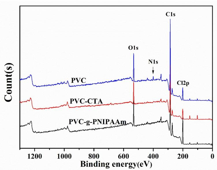
Figure S16. XPS survey spectra of PVC, PVC-CTA and PVC-g-PNIPAAm surfaces.
