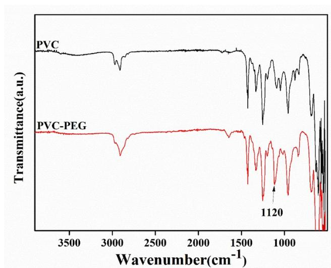
**Figure S17.** Reflectance FT-IR spectra of PVC and PVC-PEG surfaces.
