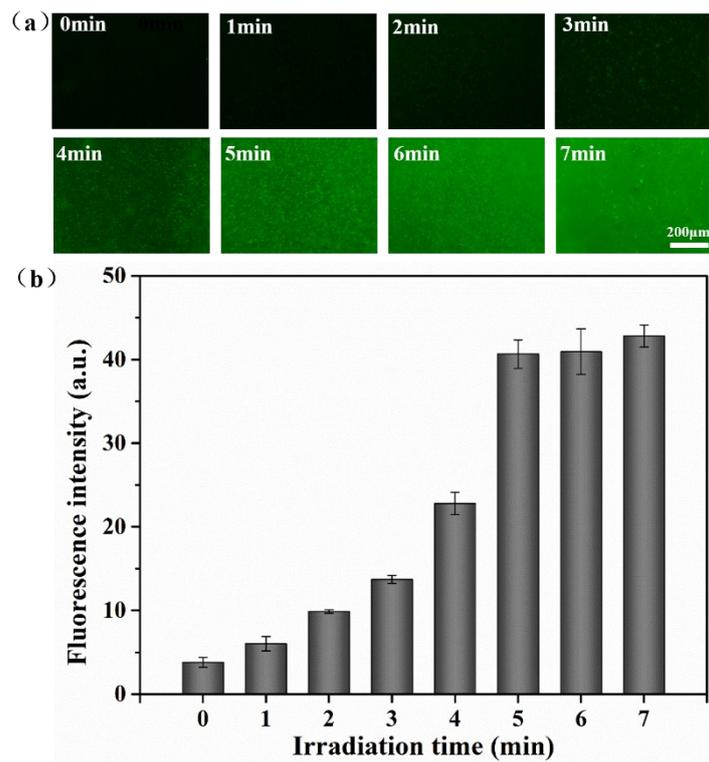
**Figure S19.** (a) Fluorescence microscopy images of the PVC-SH surfaces treated with N-(5-fluoresceinyl) maleimide in different irradiation time. (b) The fluorescence intensity of PVC-SH surfaces treated with N-(5-fluoresceinyl) maleimide in different irradiation time ( $n = 6$ ).
