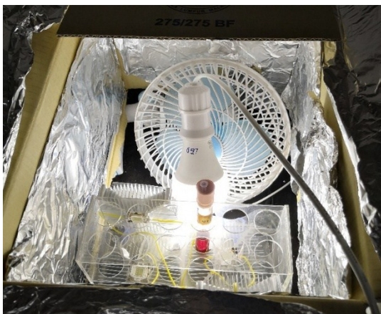
Figure S8. Homemade visible light photoreactor using a LED bulb as the light source
