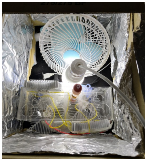
Figure S7. Homemade visible light photoreactor using a CFL bulb as the light source
