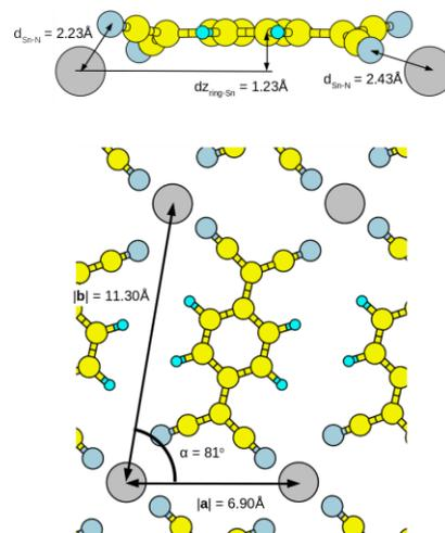
Fig. 10 Relaxed structure for an unsupported Sn-TCNQ MON.
