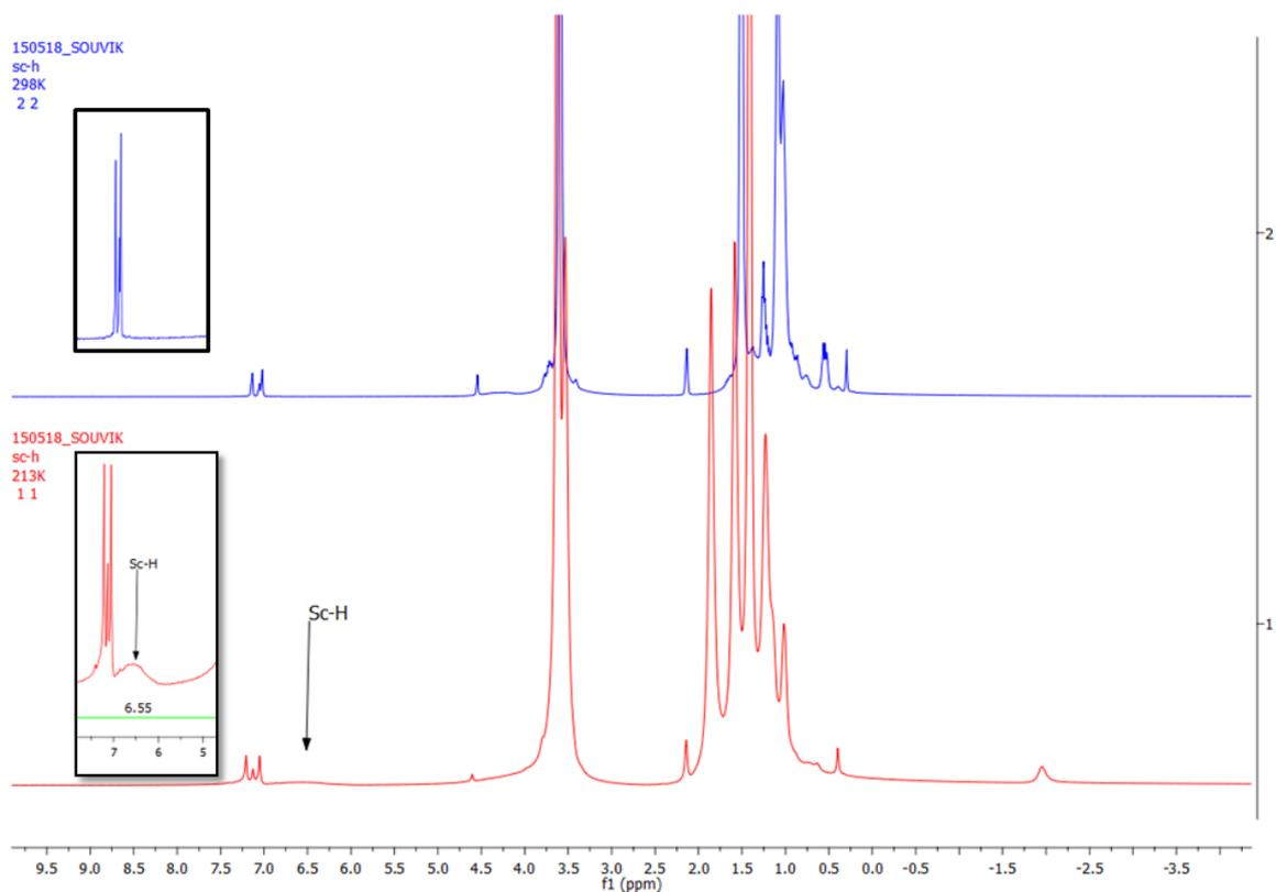
**Figure S2:** Stacked  $^1\text{H}$  NMR spectra of crude reaction mixture of  $\text{Sc}(\text{OTf})_3$  and  $\text{NaBHET}_3$  (1:1), recorded at: 1) 213 K (-60 °C); 2) 298 K.
