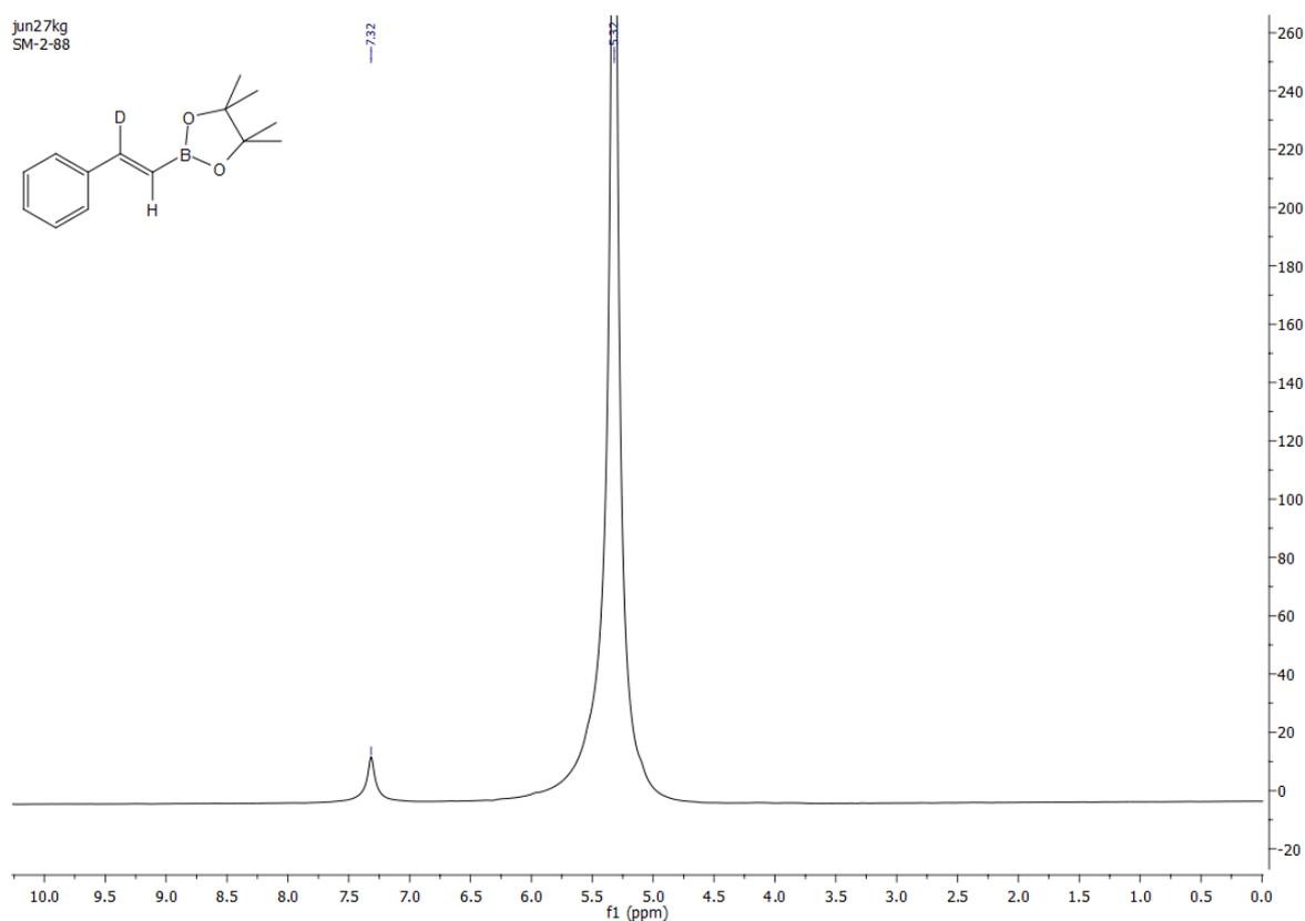
**Figure S7:** <sup>2</sup>H NMR (CD<sub>2</sub>Cl<sub>2</sub>, 62 MHz) spectra of crude reaction mixture of Sc(OTf)<sub>3</sub> + NaBHET<sub>3</sub> + **1a** + DBpin.
