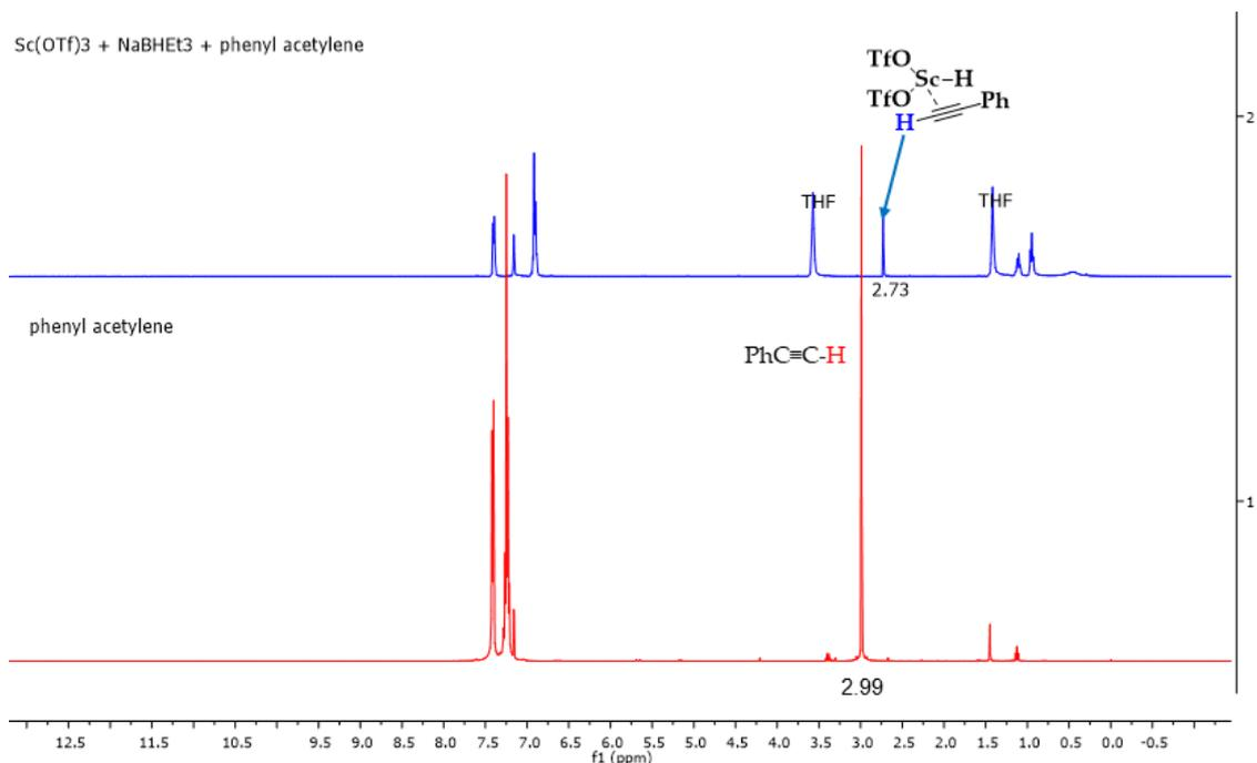
**Figure S3:** Stacked  $^1\text{H}$  NMR spectra of: 1) Phenyl acetylene (**1a**), 2)  $\text{Sc}(\text{OTf})_3 + \text{NaBHET}_3 + \text{phenyl acetylene}$  (1:1:1) (both spectra have been recorded in  $\text{C}_6\text{D}_6$ ).
