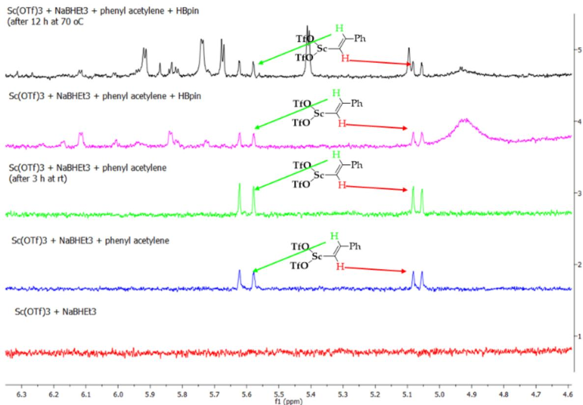
**Figure S4:** Stacked <sup>1</sup>H NMR spectra of sequential addition of reagents (expanded region from 6.3 ppm to 4.6 ppm): 1) Sc(OTf)<sub>3</sub> + NaBHET<sub>3</sub>, 2) Sc(OTf)<sub>3</sub> + NaBHET<sub>3</sub> + **1a**, 3) Sc(OTf)<sub>3</sub> + NaBHET<sub>3</sub> + **1a** (stirred at RT for 3h), 4) Sc(OTf)<sub>3</sub> + NaBHET<sub>3</sub> + **1a** + HBpin, 5) Sc(OTf)<sub>3</sub> + NaBHET<sub>3</sub> + **1a** + HBpin (after 12 h, at 70 °C).
