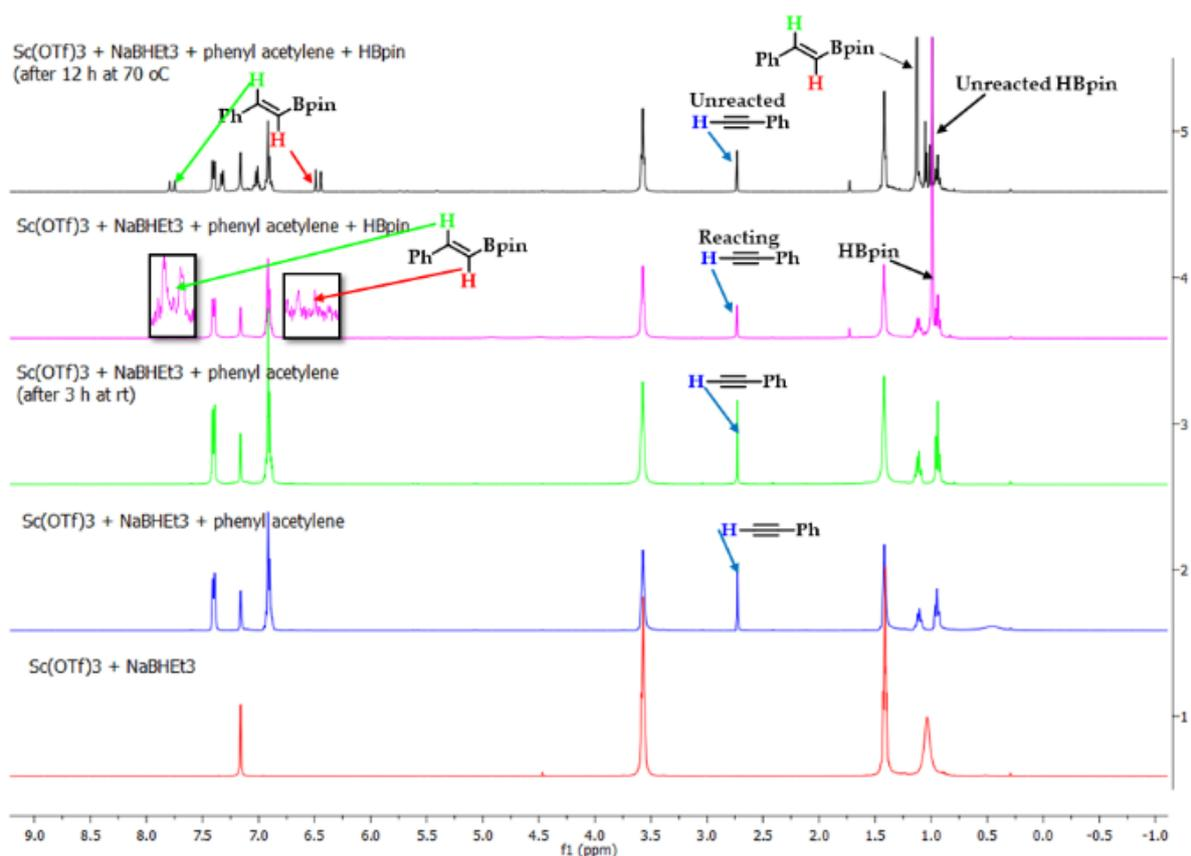
**Figure S5:** Stacked  $^1\text{H}$  NMR spectra of sequential addition of reagents: 1)  $\text{Sc}(\text{OTf})_3 + \text{NaBHET}_3$ , 2)  $\text{Sc}(\text{OTf})_3 + \text{NaBHET}_3 + \mathbf{1a}$ , 3)  $\text{Sc}(\text{OTf})_3 + \text{NaBHET}_3 + \mathbf{1a}$  (stirred at RT for 3h), 4)  $\text{Sc}(\text{OTf})_3 + \text{NaBHET}_3 + \mathbf{1a} + \text{HBpin}$ , 5)  $\text{Sc}(\text{OTf})_3 + \text{NaBHET}_3 + \mathbf{1a} + \text{HBpin}$  (after 12 h, at 70 °C).
