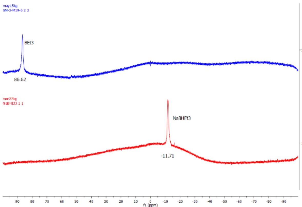
**Figure S1:**  $^{11}\text{B}$  NMR spectra of: 1)  $\text{NaBHET}_3$ , 2) Crude reaction mixture of  $\text{Sc}(\text{OTf})_3$  and  $\text{NaBHET}_3$  (1:1) at RT.
