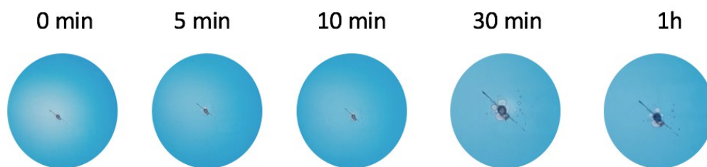
Figure S7. Control experiment for traveling wave in the absence of DMBQ. No reduction is observed over 1h period. Increase of the area of the application point can be explained by gradual degradation of the agarose gel due to spontaneous decomposition of \text{NaBH}_4 accompanied by the formation of hydrogen gas bubbles.
