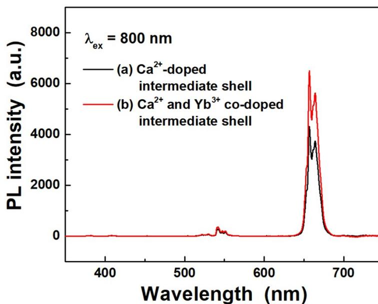
Figure S3. PL spectra of (a)  $\text{NaErF}_4:\text{Tm}(0.5\%),\text{Gd}(10\%)/\text{NaYF}_4:\text{Ca}(20\%)/\text{NaYF}_4:\text{Nd}(40\%),\text{Yb}(10\%)$  C/S/S UCNPs and (b)  $\text{NaErF}_4:\text{Tm}(0.5\%),\text{Gd}(10\%)/\text{NaYF}_4:\text{Ca}(20\%),\text{Yb}(10\%)$  / $\text{NaYF}_4:\text{Nd}(40\%),\text{Yb}(10\%)$  C/S/S UCNPs under excitation with 800 nm NIR light.
