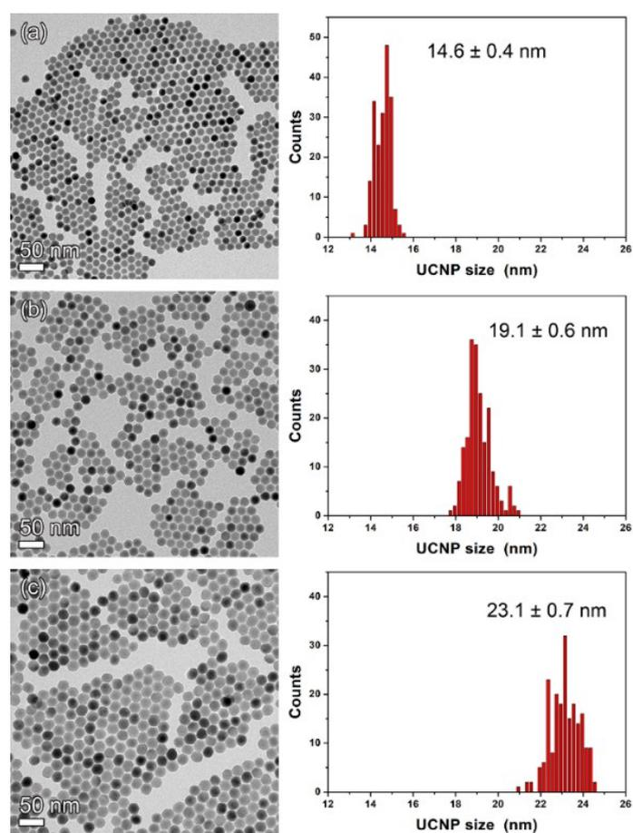
Figure S4. TEM images (left) and size distributions (right) of (a) NaErF<sub>4</sub>:Tm(0.5%),Gd(10%) core UCNPs, (b) NaErF<sub>4</sub>:Tm(0.5%),Gd(10%)/NaYF<sub>4</sub>:Ca(20%),Yb(10%) C/S UCNPs, and (c) NaErF<sub>4</sub>:Tm(0.5%),Gd(10%)/NaYF<sub>4</sub>:Ca(20%),Yb(10%)/NaYF<sub>4</sub>:Nd(40%),Yb(10%) C/S/S UCNPs.
