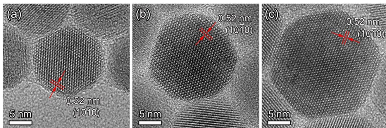
Figure S5. HR-TEM images of (a)  $\text{NaErF}_4:\text{Tm}(0.5\%),\text{Gd}(10\%)$  core UCNPs, (b)  $\text{NaErF}_4:\text{Tm}(0.5\%),\text{Gd}(10\%)/\text{NaYF}_4:\text{Ca}(20\%),\text{Yb}(10\%)$  C/S UCNPs, and (c)  $\text{NaErF}_4:\text{Tm}(0.5\%),\text{Gd}(10\%)/\text{NaYF}_4:\text{Ca}(20\%),\text{Yb}(10\%)/\text{NaYF}_4:\text{Nd}(40\%),\text{Yb}(10\%)$  C/S/S UCNPs.
