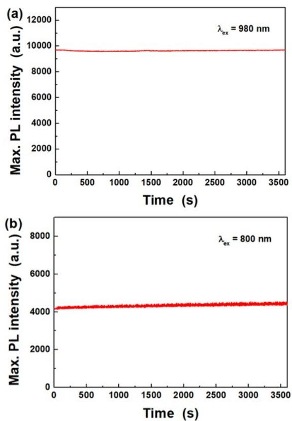
Figure S9. Maximum PL intensities of the NaErF<sub>4</sub>:Tm(0.5%),Gd(10%)/NaYF<sub>4</sub>:Ca(20%),Yb(10%)/NaYF<sub>4</sub>:Nd(40%),Yb(10%) C/S/S UCNP<sub>s</sub> under continuous irradiations with (a) 980 nm and (b) 800 nm NIR lasers (laser power = 2 W).
