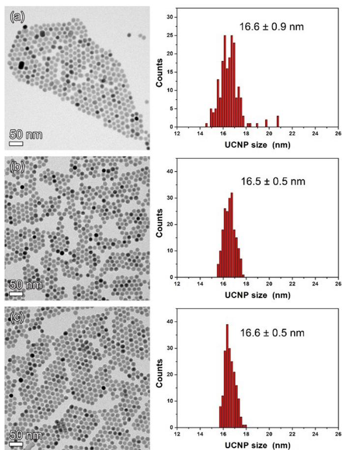
Figure S2. TEM images (left) and size distributions (right) of (a) NaErF<sub>4</sub>:Tm(0.5%),Gd(10%)/NaYF<sub>4</sub> C/S UCNPs, (b) NaErF<sub>4</sub>:Tm(0.5%),Gd(10%)/NaYF<sub>4</sub>:Ca(20%) C/S UCNPs, and (c) NaErF<sub>4</sub>:Tm(0.5%),Gd(10%)/NaYF<sub>4</sub>:Nd(20%) C/S UCNPs.
