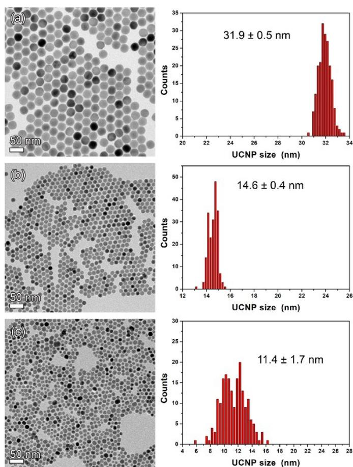
Figure S1. TEM images (left) and size distributions (right) of (a) NaErF<sub>4</sub>:Tm(0.5%) UCNPs, (b) NaErF<sub>4</sub>:Tm(0.5%),Gd(10%) UCNPs, and (c) NaErF<sub>4</sub>:Tm(0.5%),Gd(30%) UCNPs.
