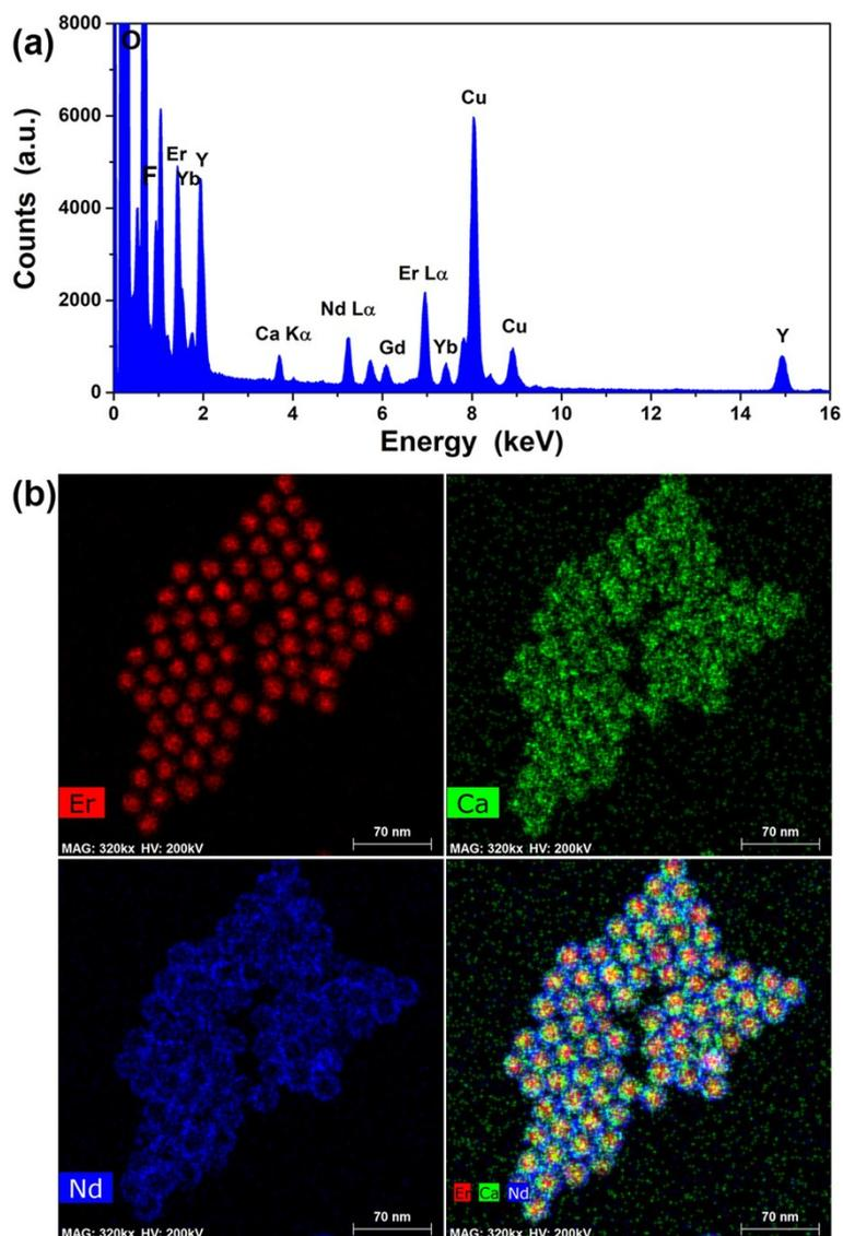
Figure S6. (a) EDS spectrum and (b) EDS maps for NaErF<sub>4</sub>:Tm(0.5%),Gd(10%)/NaYF<sub>4</sub>:Ca(20%),Yb(10%)/NaYF<sub>4</sub>:Nd(40%),Yb(10%) C/S/S UCNPs. The composite EDS map was generated by superposing Er L $\alpha$  map (red), Ca K $\alpha$  map (green), and Nd L $\alpha$  map (blue).
