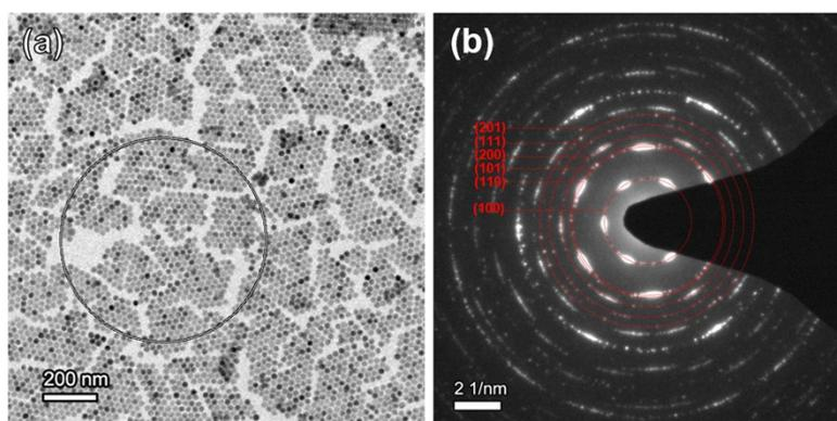
Figure S7. (a) TEM image and (b) selected area electron diffraction (SAED) pattern of the C/S/S UCNPs. The SAED pattern was obtained for the area indicated with a solid circle in the TEM image.
