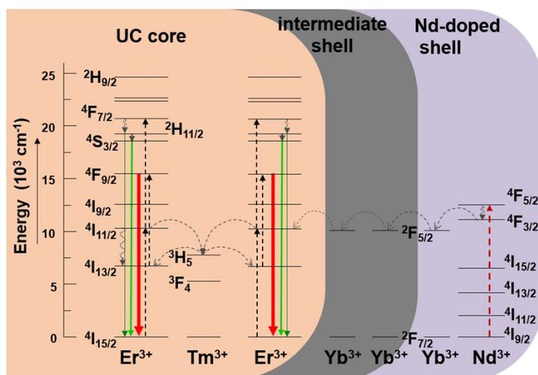
Figure S8. Schematic energy level diagram showing UC luminescence mechanism of the  $\text{NaErF}_4:\text{Tm}(0.5\%),\text{Gd}(10\%)/\text{NaYF}_4:\text{Ca}(20\%),\text{Yb}(10\%)/\text{NaYF}_4:\text{Nd}(40\%),\text{Yb}(10\%)$  C/S/S UCNPs.
