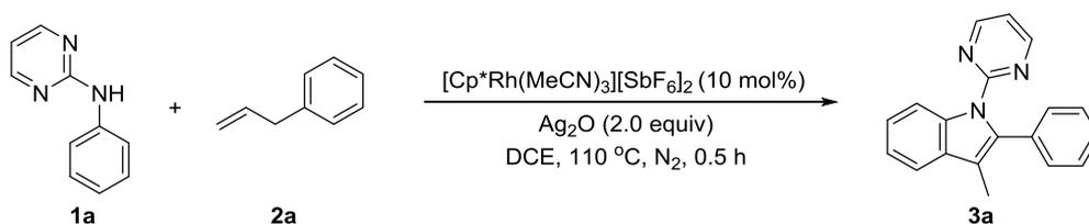
An oven-dried Schlenk tube with a magnetic stir bar was charged with  $[Cp^*Rh(MeCN)_3][SbF_6]_2$  (0.02 mmol, 16.6 mg),  $Ag_2O$  (0.4 mmol, 92.7 mg), *N*-phenylpyrimidin-2-amine **1a** (0.2 mmol, 34.2 mg) and DCE (1.0 mL) under an  $N_2$  atmosphere. Then allylbenzene **2a** (0.3 mmol, 40  $\mu$ L) was added. The resulting mixture was stirred at room temperature for 5 min and then stirred at 110  $^\circ$ C for 0.5 h. Then the HRMS analysis of the resultant solution was subsequently performed.
