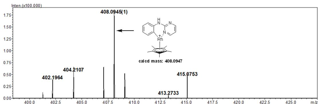
**Figure S3.** HRMS (ESI<sup>+</sup>) spectrum of intermediate **A**, calcd. 408.0947, found 408.0945.
