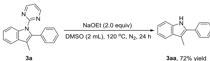
**Scheme S4.** Procedure for the removal of the directing group.
