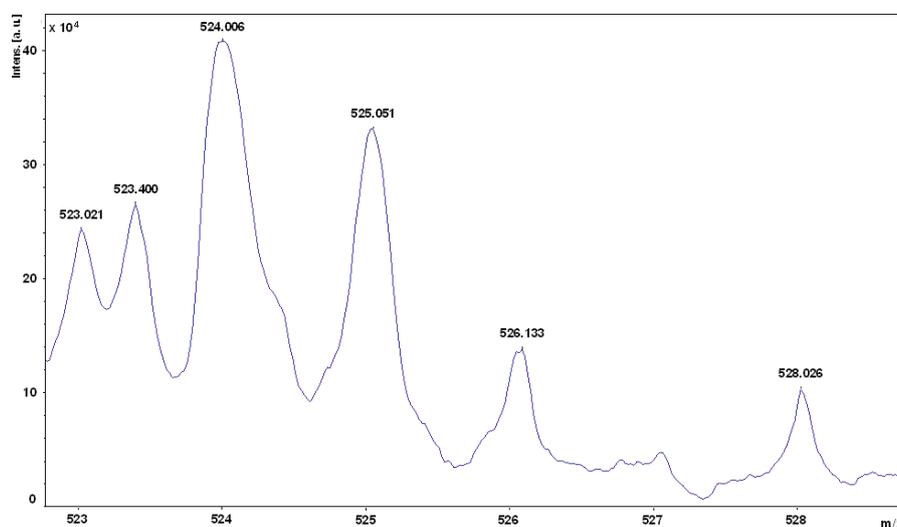
**Figure S1.** Matrix-assisted laser desorption ionization time-of-flight mass spectroscopy (MALDI-TOF-MS) of intermediate **B** or **C** (calcd. mass 525.165, found 525.051).
