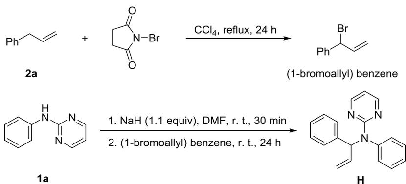
**Scheme S3.** General procedure for the synthesis of *N*-phenyl-*N*-(1-phenylallyl)pyrimidin-2-amine **H**.
