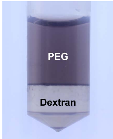
Fig. S2 Optical image of aqueous PEG and dextran biphasic solutions. The purple color of the PEG phase indicates that TA in the dextran phase moved into the PEG phase.
