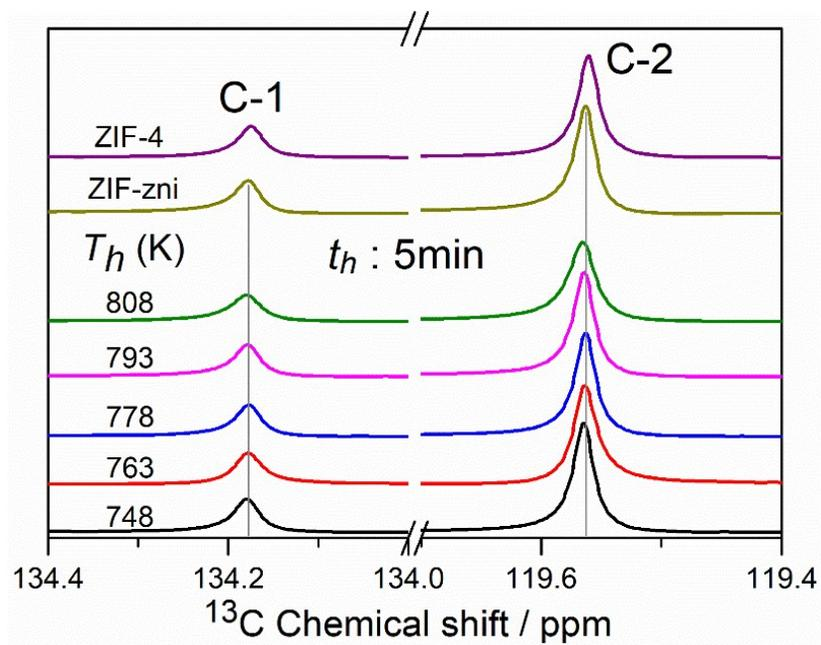
**Figure S6.** An enlarged area of  $^{13}\text{C}$  LS-NMR spectra of ZIF-4, ZIF-zni and fq-agZIF-4 heat-treated at 748, 763, 778, 793 and 808 K for 5 mins.
