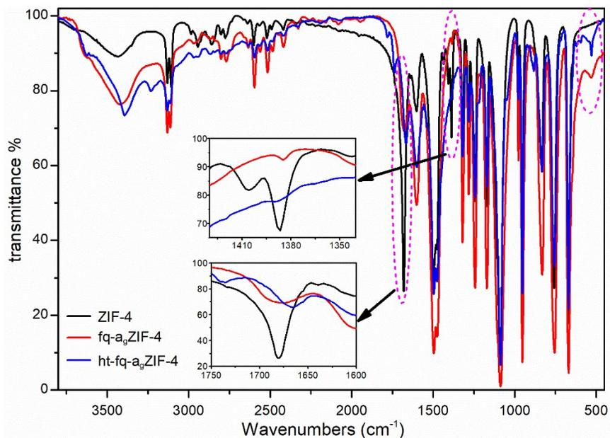
**Figure S7.** FT-IR absorption curves in KBr of ZIF-4, fq-a<sub>9</sub>ZIF-4 and ht-fq-a<sub>9</sub>ZIF-4. The magenta circles marked the main changed areas. Inset: enlarged images of the chosen areas.
