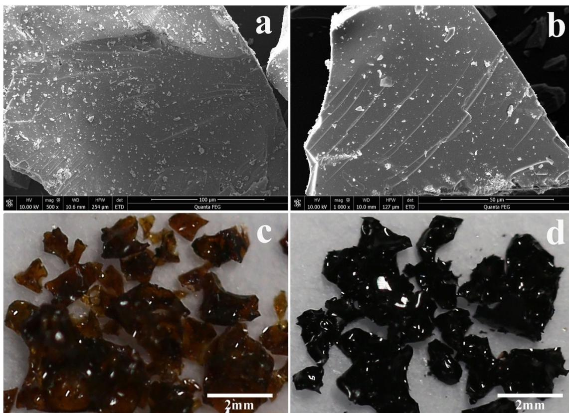
**Figure S4.** SEM images of (a) fq-a<sub>6</sub>ZIF-4 and (b) ht-fq-a<sub>6</sub>ZIF-4. Optical images of (c) fq-a<sub>6</sub>ZIF-4 and (d) ht-fq-a<sub>6</sub>ZIF-4.
