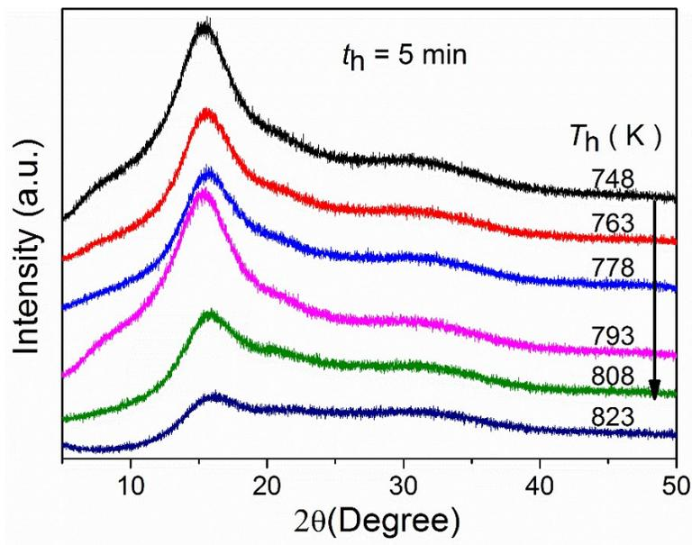
**Figure S1.** PXRD patterns of the fq-a<sub>g</sub>ZIF-4 heat-treated at various values of T<sub>h</sub> for 5 min.
