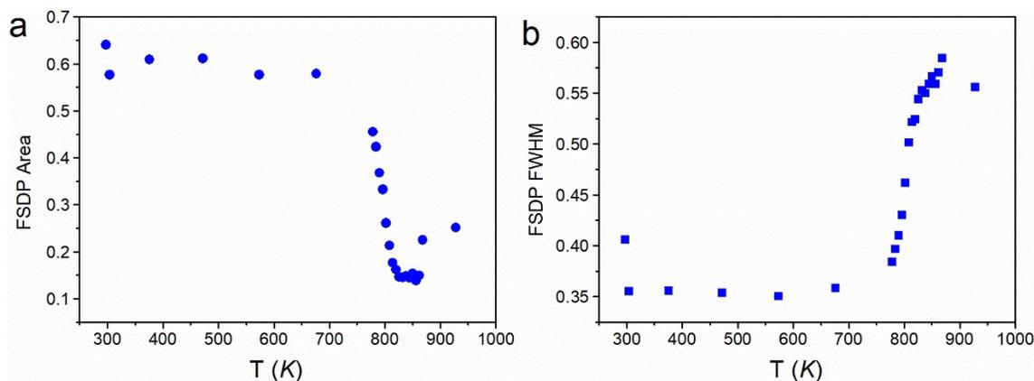
**Figure S9.** Variable temperature synchrotron X-ray total scattering data  $S(Q)$ . Variance in the (a) area and (b) FWHM of the first sharp diffraction peak (FSDP) with temperature.
