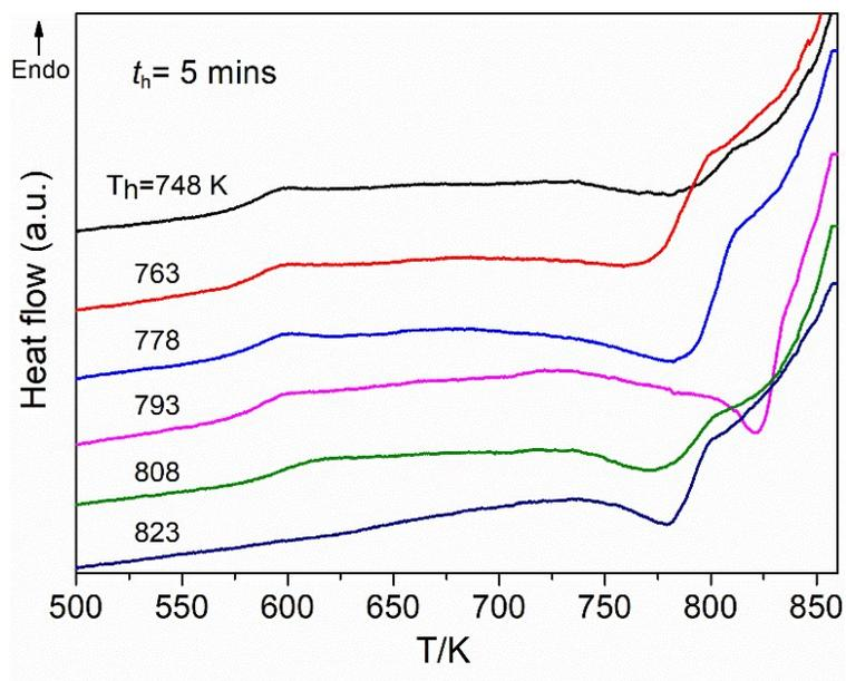
**Figure S2.** DSC experiments on the fq-a<sub>g</sub>ZIF-4 heat-treated at various values of T<sub>h</sub> for 5 min.
